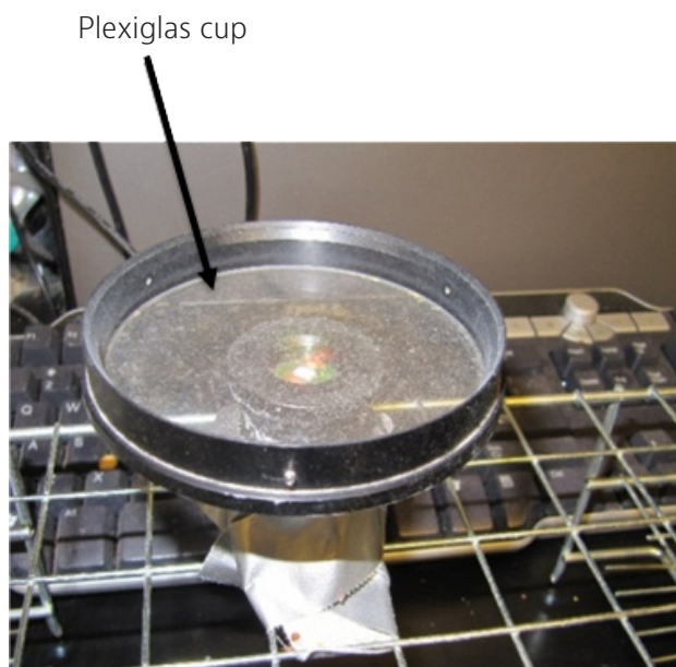
Figure 2. An empty Plexiglas cup with a MicroNIR spectrometer positioned below the plastic surface of the cup
