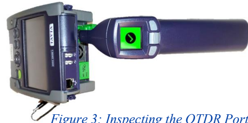
Figure 3: Inspecting the OTDR Port
