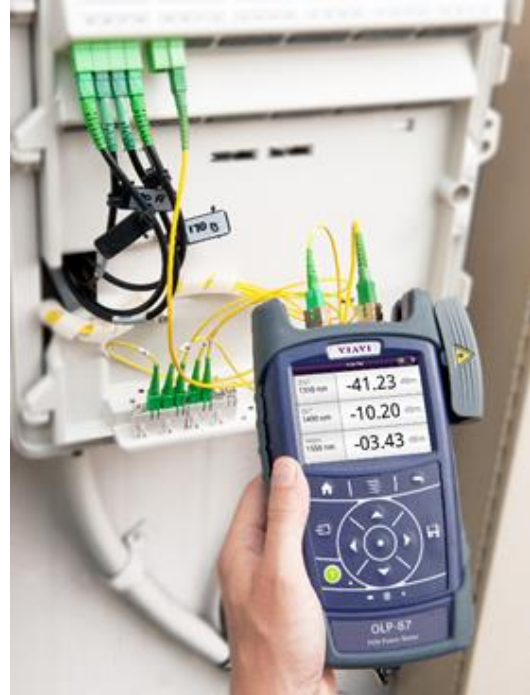
Figure 5: Through Mode testing
