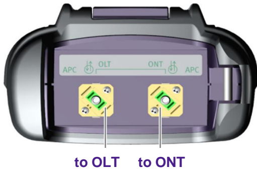
Figure 4: OL-87, Top View (Power Meter Connectors)
