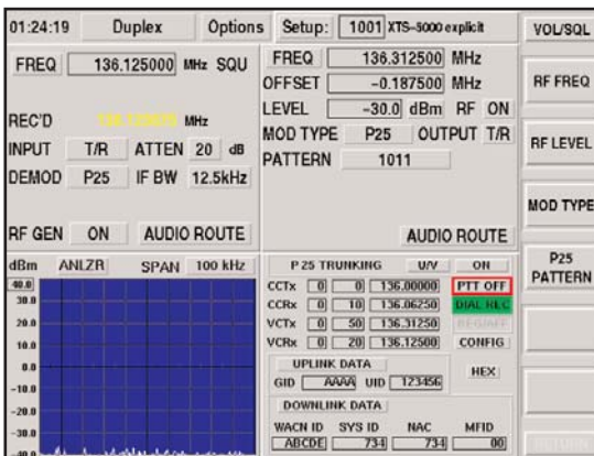
Figure 46: The 2975 Displaying the Dial Request Received from the SU during a PSTN Dial Call
