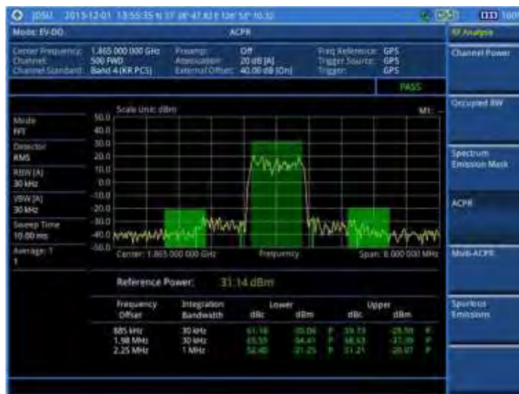
Figure 174 ACPR measurement with EV-DO signal analyzer
