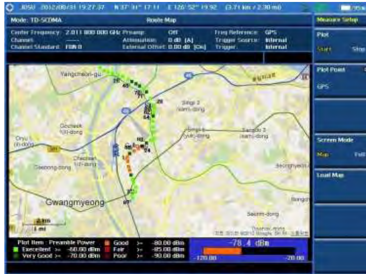
Figure 214 Route map measurement with TD-SCDMA OTA signal analyzer
