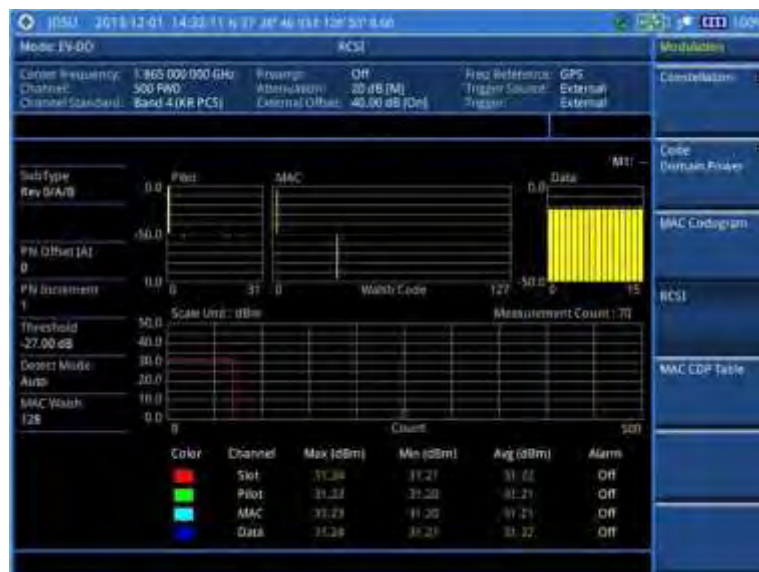
Figure 182 RCSI measurement with EV-DO signal analyzer
