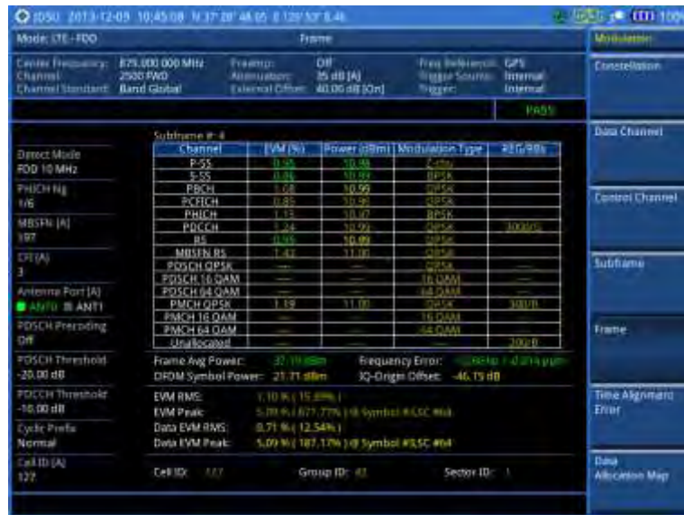
Figure 93 Frame measurement with LTE - FDD signal analyzer (MBMS On)
