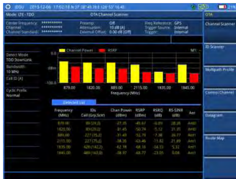
Figure 136 Channel scanner measurement with LTE - TDD OTA signal analyzer
