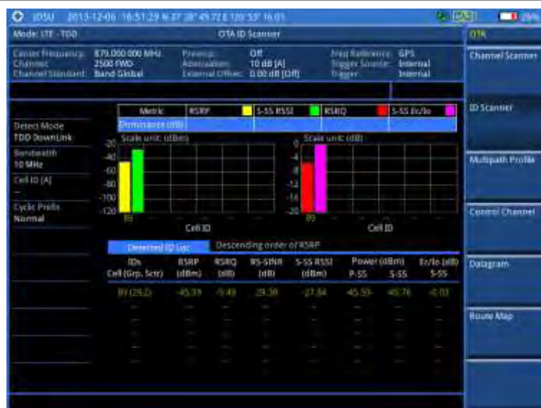
Figure 137 ID scanner measurement with LTE - TDD OTA signal analyzer
