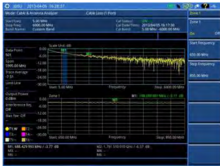
Figure 248 Cable loss (1 port) measurement with the zone enabled
