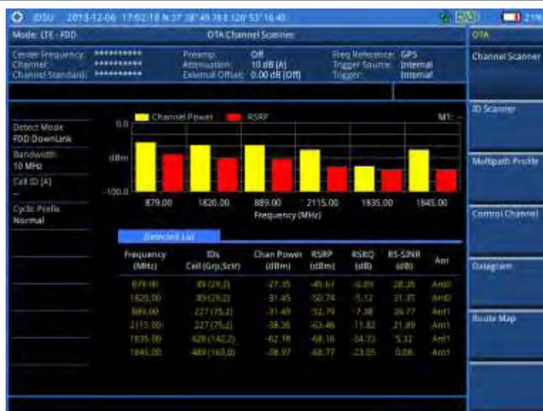
Figure 101 Channel scanner measurement with LTE - FDD OTA signal analyzer
