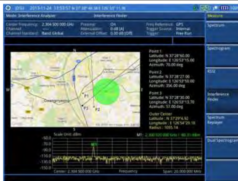
Figure 28 Interference finder measurement in map view
