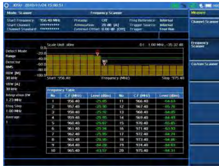
Figure 271 Frequency scanner measurement
