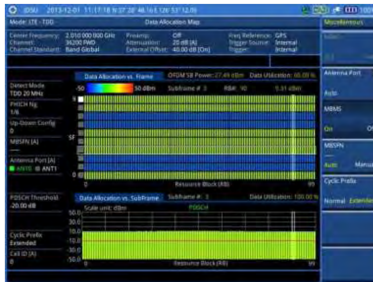
Figure 131 Data allocation map measurement with LTE - TDD signal analyzer (MBMS On)
