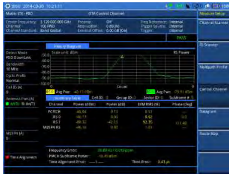
Figure 104 Control channel measurement with LTE - FDD OTA signal analyzer
