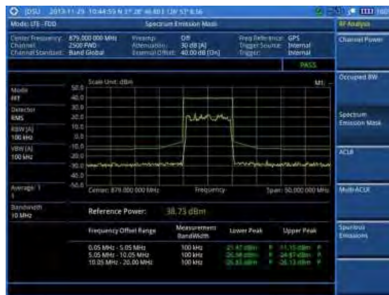
Figure 79 SEM measurement with LTE - FDD signal analyzer
