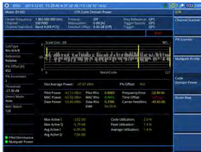
Figure 188 Code domain power measurement with EV-DO OTA signal analyzer
