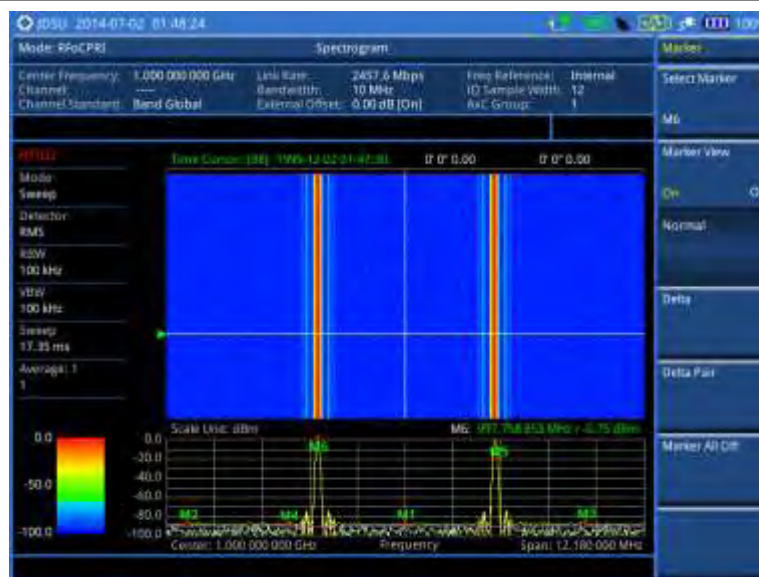
Figure 262 RFoCPRI interference measurement in spectrogram
