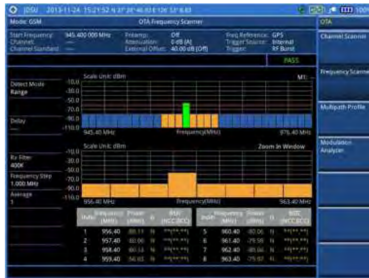
Figure 44 Frequency scanner measurement with GSM OTA signal analyzer
