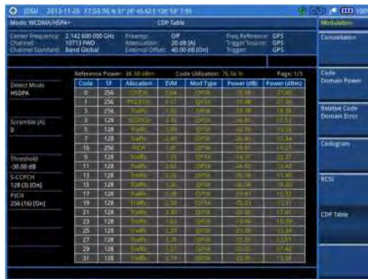
Figure 64 CDP Table measurement with WCDMA/HSPA+ signal analyzer
