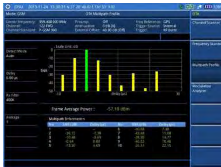
Figure 45 Multipath profile measurement with GSM OTA signal analyzer
