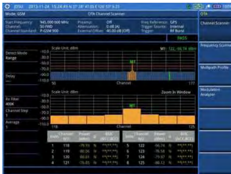
Figure 43 Channel scanner measurement with GSM OTA signal analyzer
