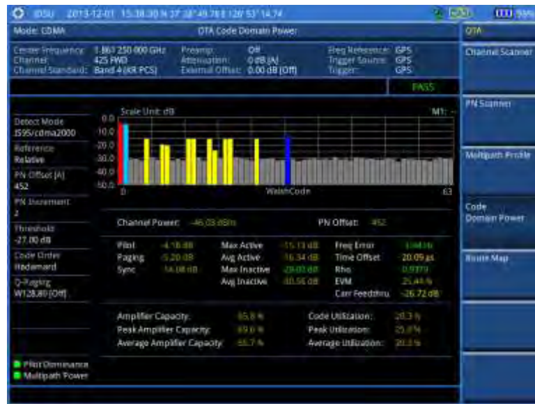
Figure 163 Code domain power measurement with CDMA OTA signal analyzer
