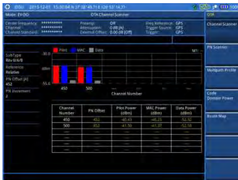
Figure 185 Channel scanner measurement with EV-DO OTA signal analyzer
