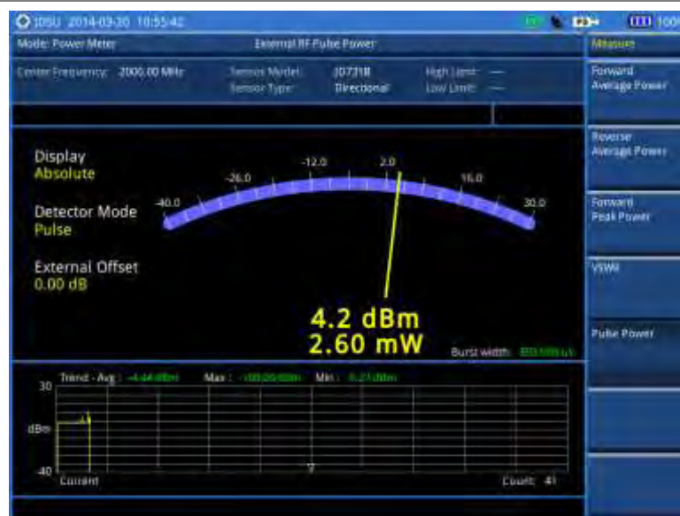
Figure 278 External power measurement of pulse power
