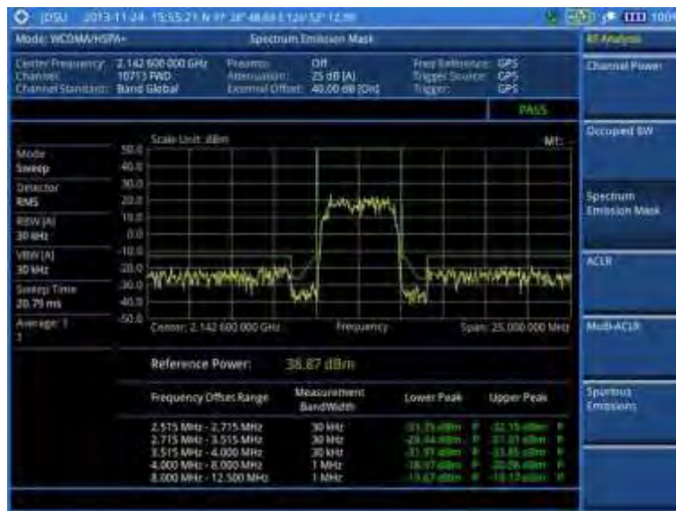
Figure 55 SEM measurement with WCDMA/HSPA+ signal analyzer
