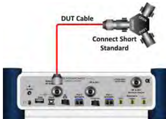
Figure 240 Connection for cable loss (1 port) measurement
