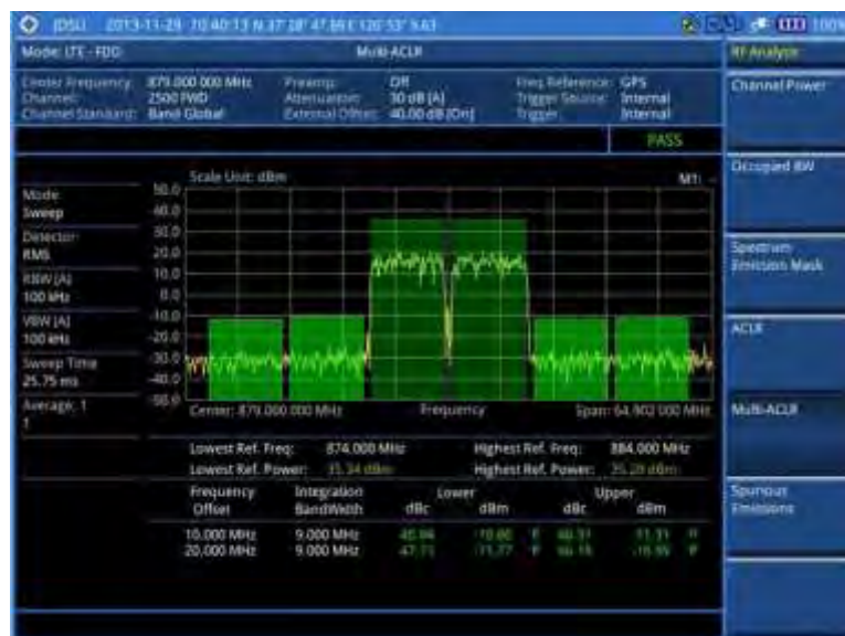
Figure 81 Multi-ACLR measurement with LTE - FDD signal analyzer
