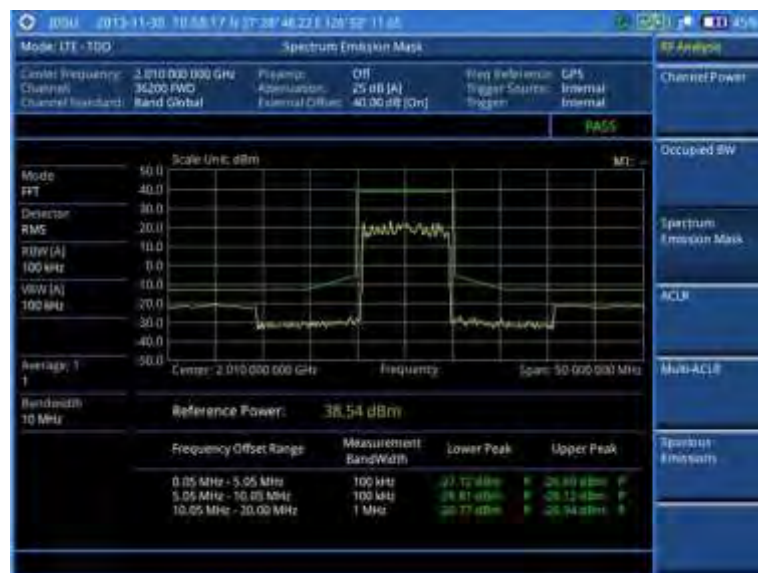
Figure 115 SEM measurement with LTE - TDD signal analyzer
