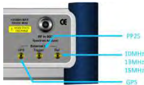
Figure 169 Connection ports for external reference clock
