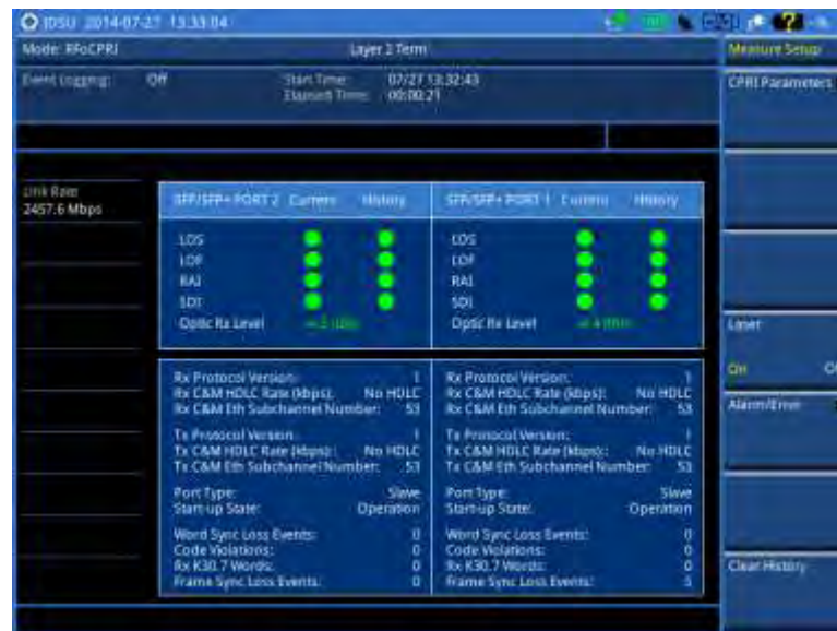
Figure 258 CPRI layer 2 term test as slave
