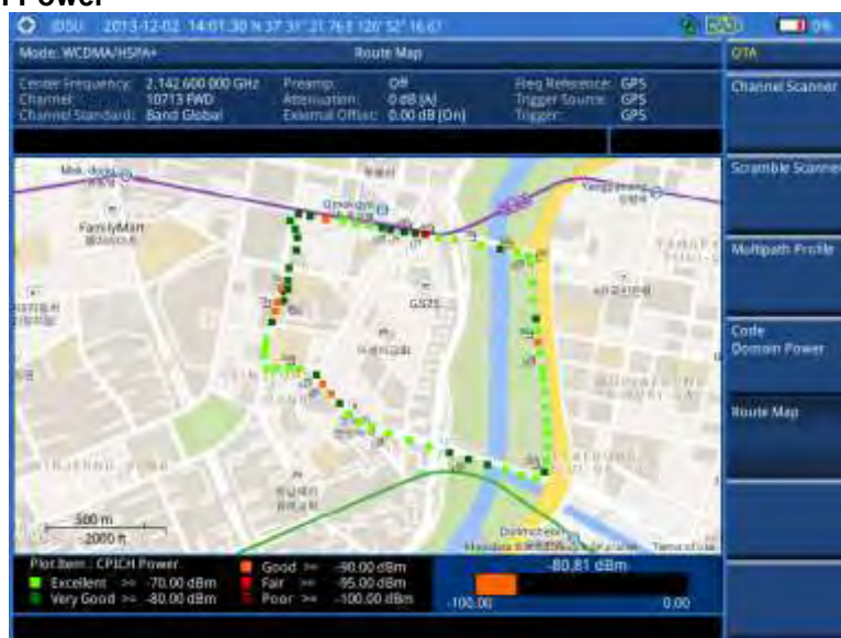
Figure 70 Route map measurement with WCDMA/HSPA+ OTA signal analyzer
