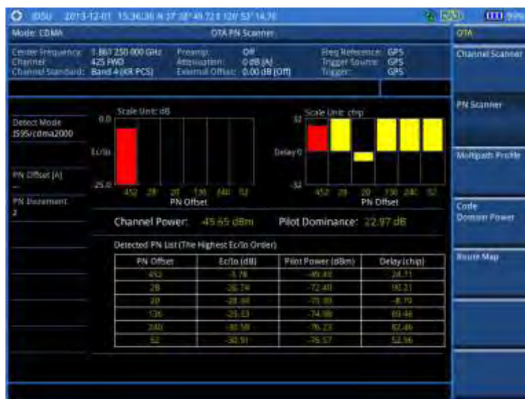
Figure 161 PN scanner measurement with CDMA OTA signal analyzer
