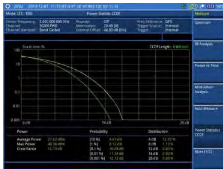
Figure 133 CCDF measurement with LTE - TDD signal analyzer
