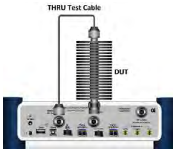
Figure 241 Connection for 2-port vector measurement
