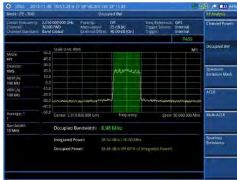
Figure 114 Occupied bandwidth measurement with LTE - TDD signal analyzer
