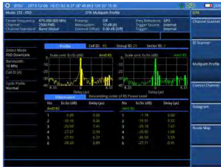
Figure 103 Multipath profile measurement with LTE - FDD OTA signal analyzer
