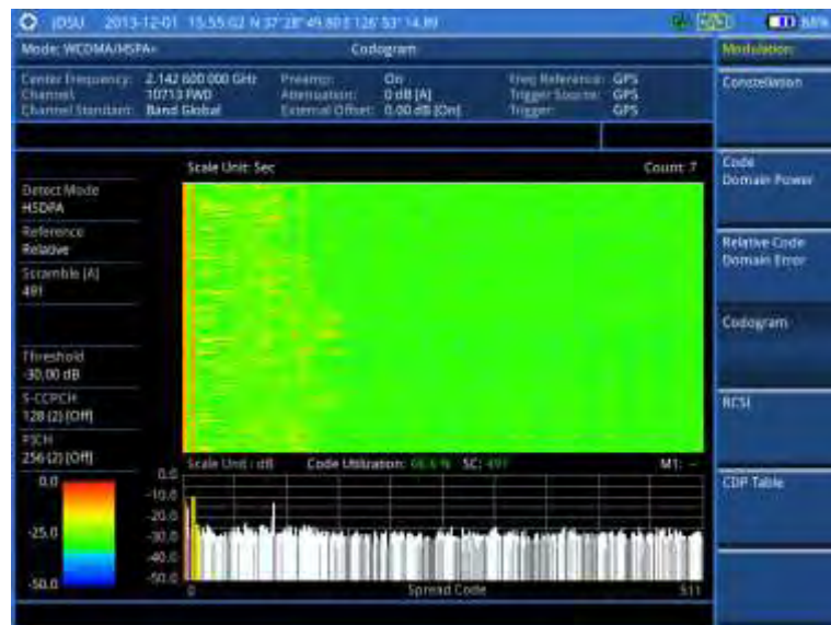
Figure 62 Codogram in full view with WCDMA/HSPA+ signal analyzer
