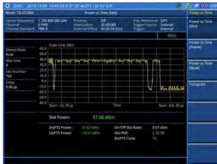
Figure 202 Power vs. time (slot) measurement with TD-SCDMA signal analyzer
