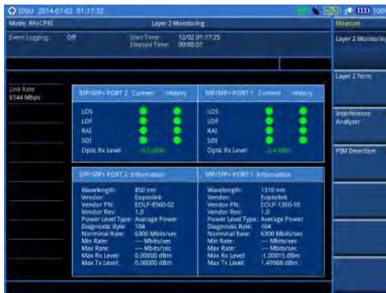
Figure 256 CPRI layer 2 monitoring
