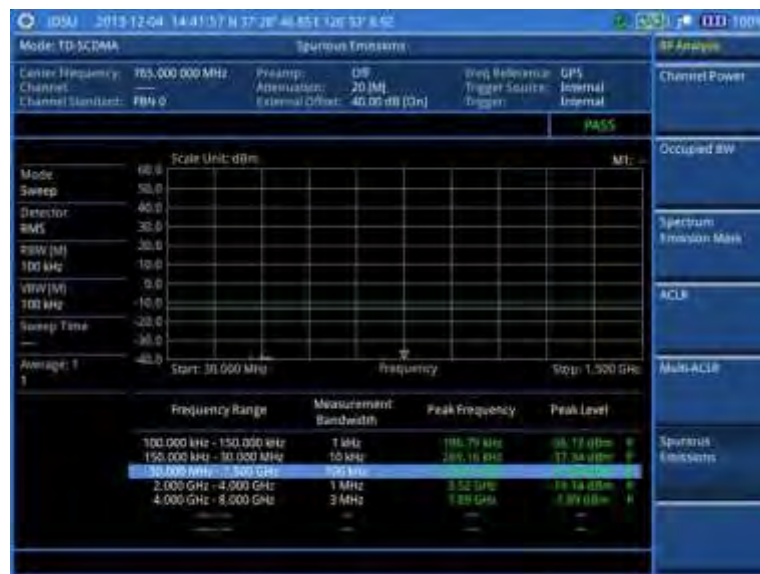
Figure 201 Spurious emissions measurement with TD-SCDMA signal analyzer
