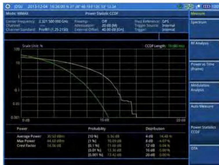
Figure 230 CCDF measurement with Mobile WiMAX signal analyzer
