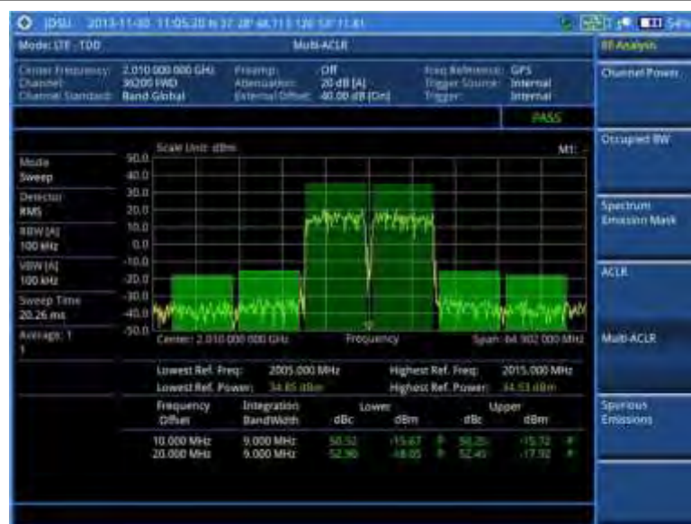
Figure 117 Multi-ACLR measurement with LTE - TDD signal analyzer
