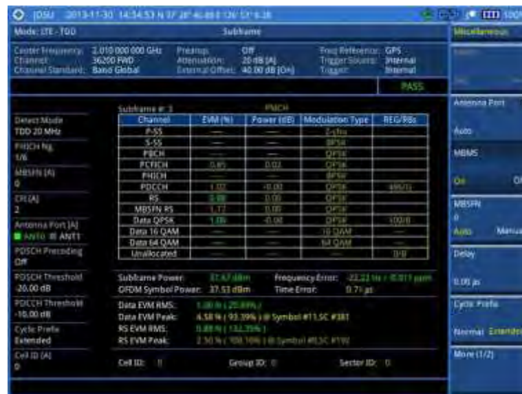
Figure 128 Subframe measurement with LTE - TDD signal analyzer (MBMS On)
