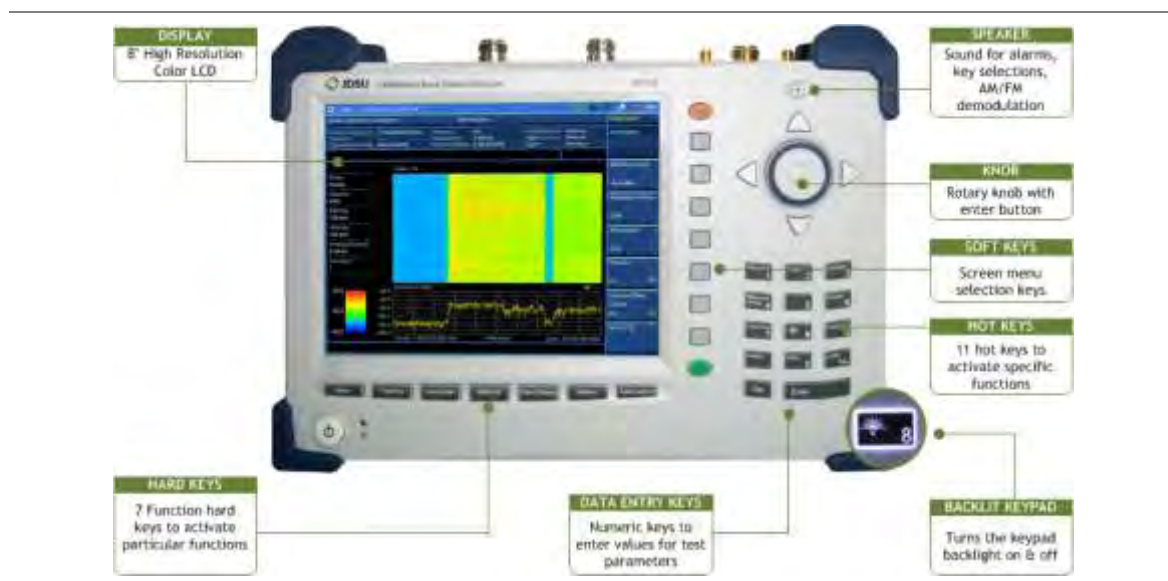
Figure 1 JD785B front panel view
