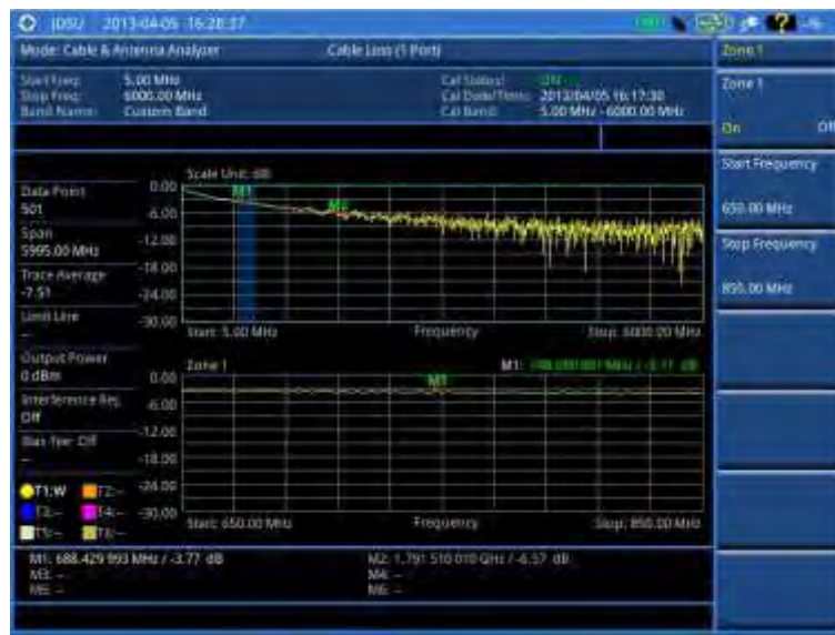
Figure 250 Cable loss (1 port) measurement with zoom
