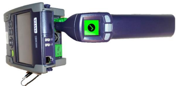
Figure 3: OTDR Port Inspection
