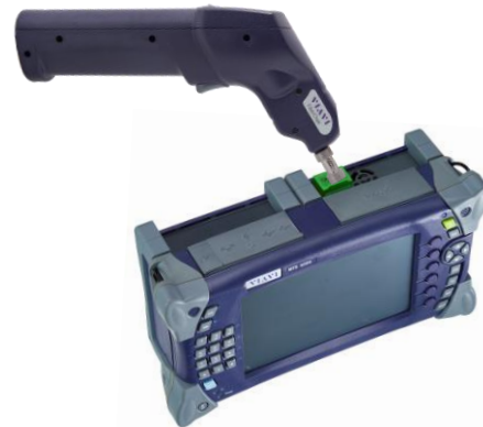
Figure 3: OTDR Port Inspection
