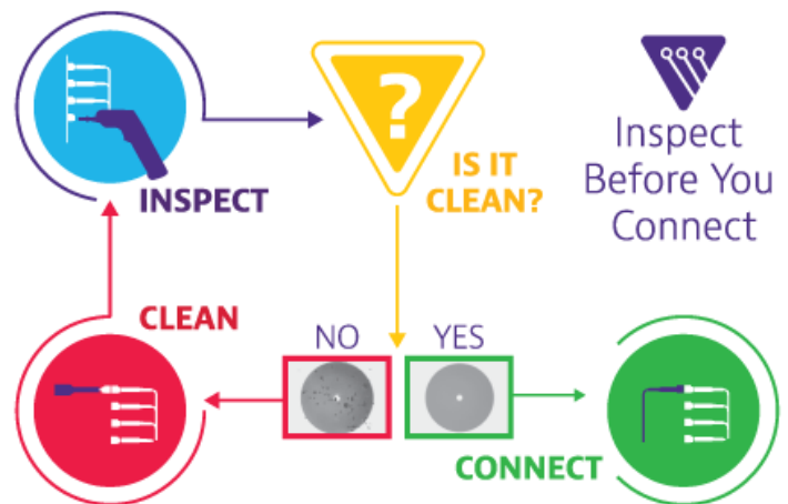
Figure 2: Inspect Before You Connect
