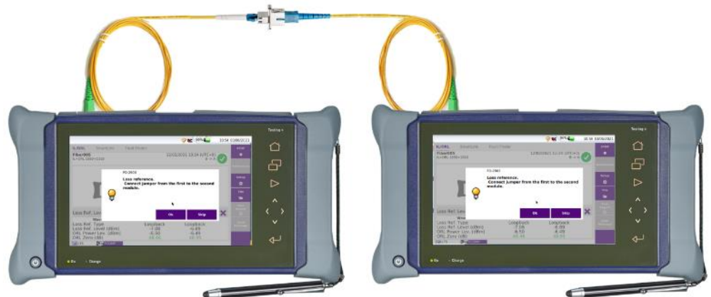
Figure 9: “Two-cable” Side-by-Side Reference
