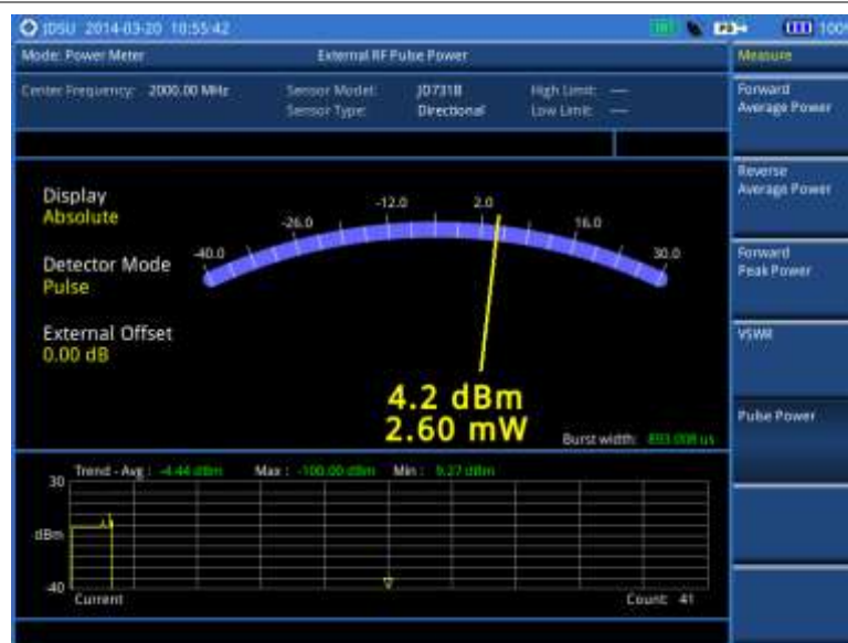
Figure 277 External power measurement of pulse power
