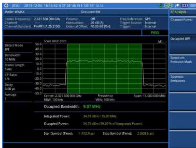
Figure 218 Occupied bandwidth measurement with Mobile WiMAX signal analyzer
