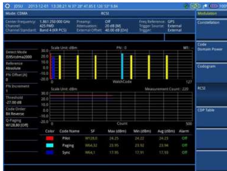
Figure 153 RCSI measurement with CDMA signal analyzer
