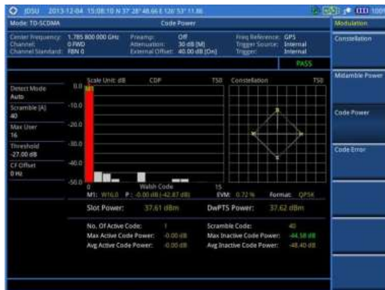
Figure 204 Code power measurement with TD-SCDMA signal analyzer
