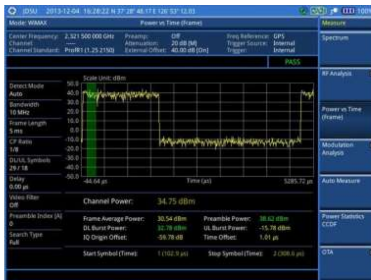
Figure 221 Power vs. time (frame) measurement with Mobile WiMAX signal analyzer
