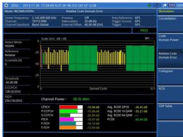
Figure 57 Relative code domain error with WCDMA/HSPA+ signal analyzer
