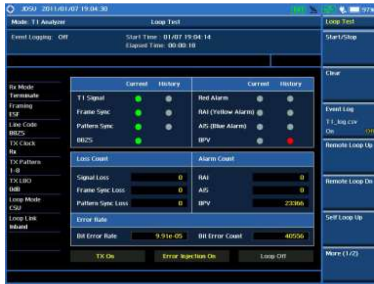
Figure 264 T1 loop testing
