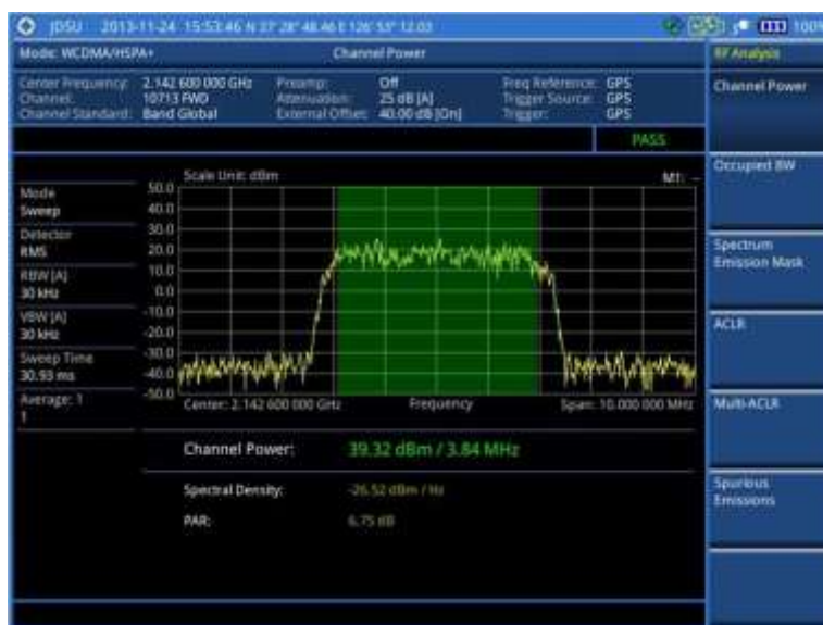
Figure 49 Channel power measurement with WCDMA/HSPA+ signal analyzer
