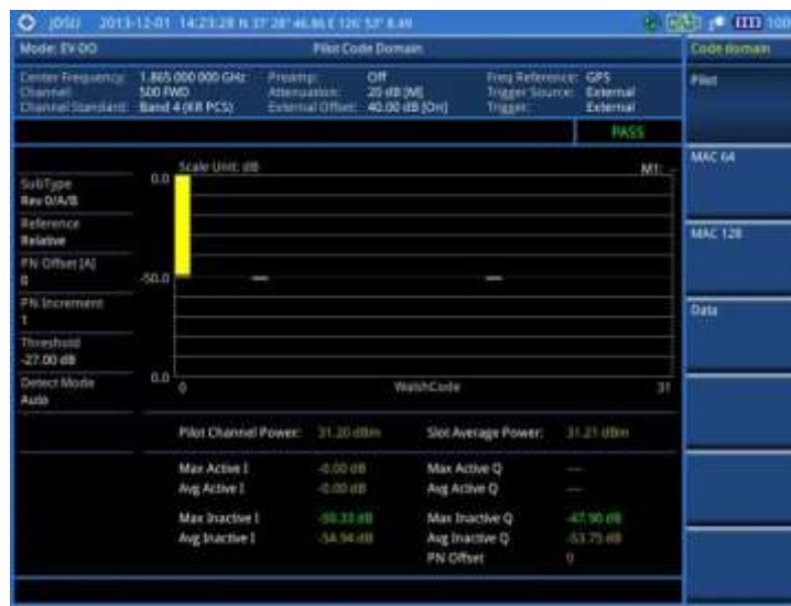
Figure 176 Code domain power measurement with EV-DO signal analyzer
