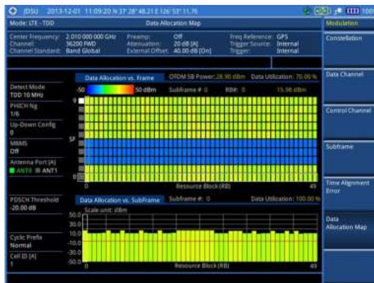
Figure 126 Data allocation map measurement with LTE - TDD signal analyzer
