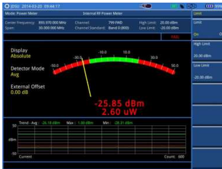
Figure 275 Internal power measurement
