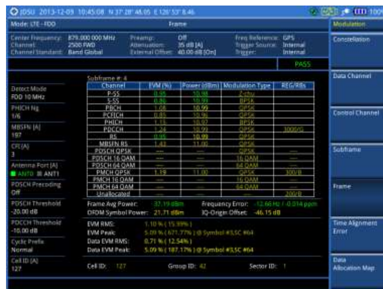
Figure 89 Frame measurement with LTE - FDD signal analyzer (MBMS On)
