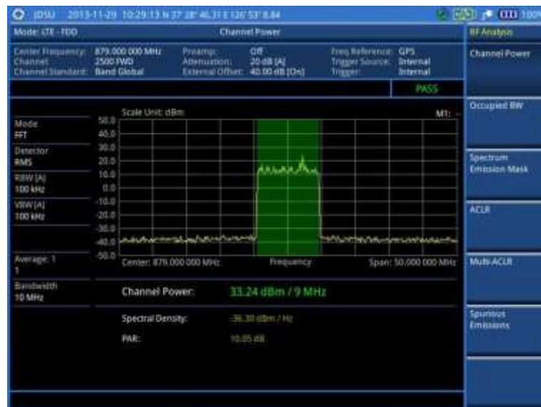
Figure 73 Channel power measurement with LTE - FDD signal analyzer
