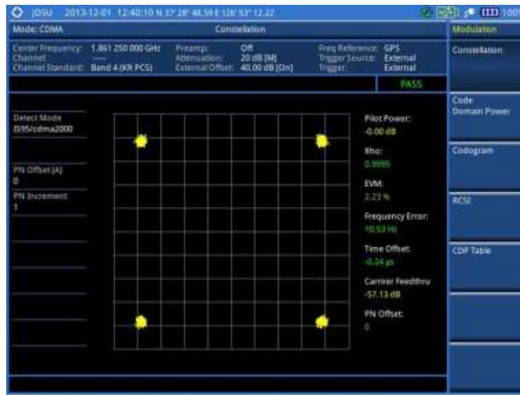
Figure 150 Constellation measurement with CDMA signal analyzer
