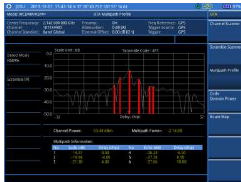
Figure 64 Multipath profile measurement with WCDMA/HSPA+ OTA signal analyzer
