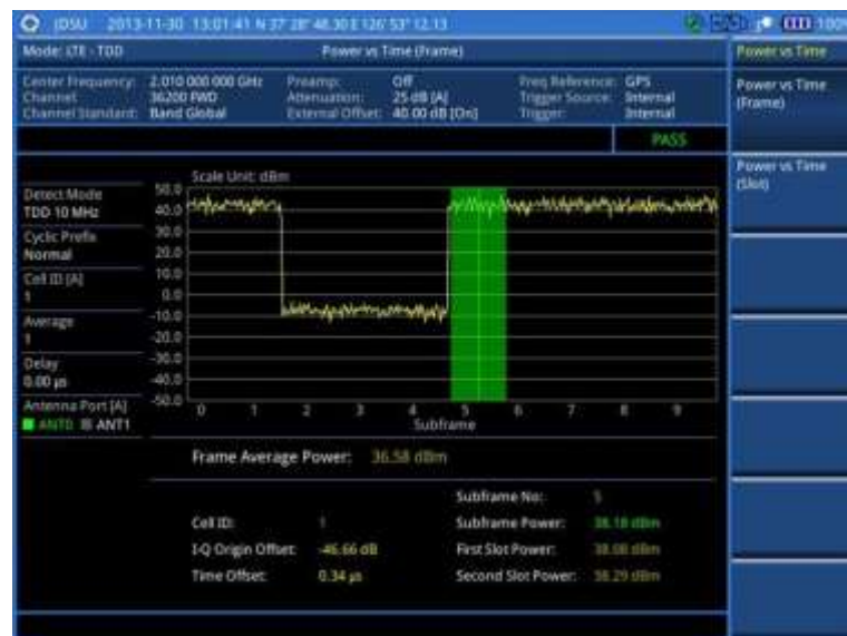
Figure 116 Power vs. time (frame) measurement with LTE – TDD signal analyzer
