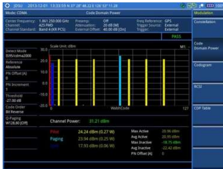
Figure 151 Code domain power measurement with CDMA signal analyzer
