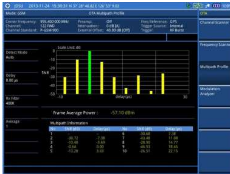
Figure 41 Multipath profile measurement with GSM OTA signal analyzer
