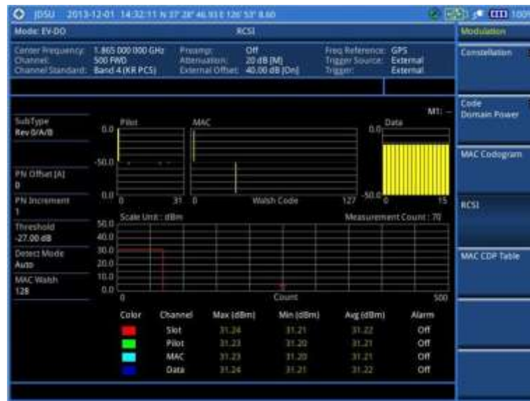
Figure 178 RCSI measurement with EV-DO signal analyzer
