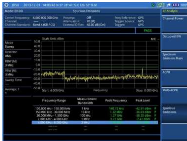
Figure 172 Spurious emissions measurement with EV-DO signal analyzer
