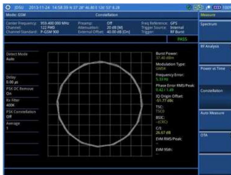
Figure 38 Constellation measurement with GSM signal analyzer
