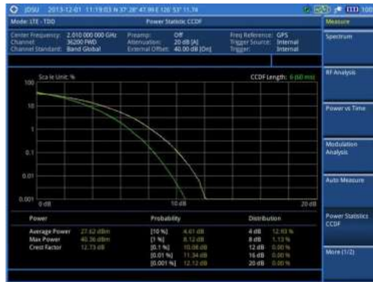
Figure 129 CCDF measurement with LTE - TDD signal analyzer
