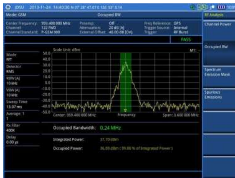
Figure 33 Occupied bandwidth measurement with GSM signal analyzer
