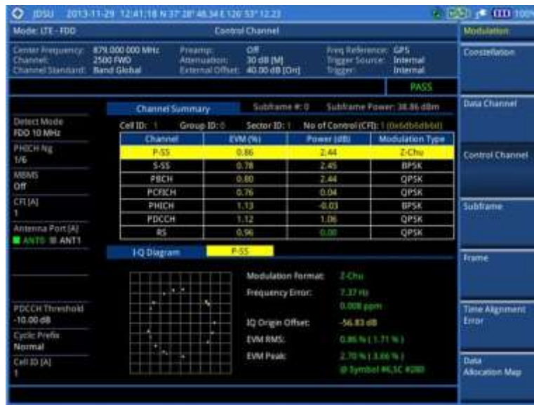
Figure 85 Control channel measurement with LTE - FDD signal analyzer (MBMS On)
