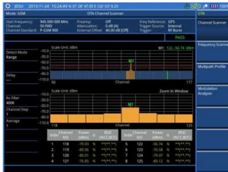
Figure 39 Channel scanner measurement with GSM OTA signal analyzer
