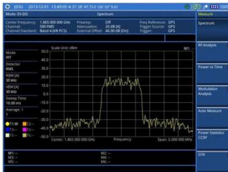
Figure 166 Spectrum measurement screen with EV-DO signal analyzer
