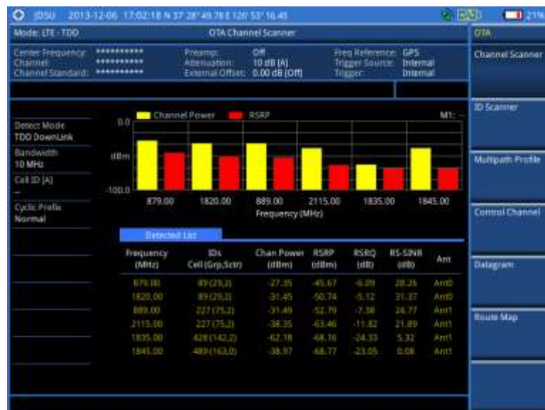
Figure 132 Channel scanner measurement with LTE - TDD OTA signal analyzer
