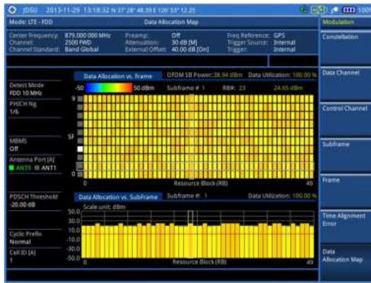
Figure 92 Data allocation map measurement with LTE - FDD signal analyzer (MBMS On)
