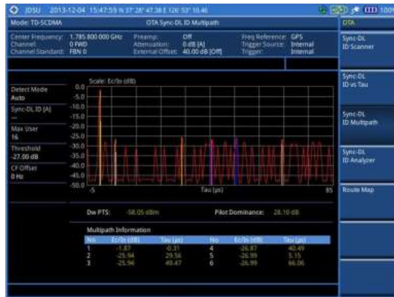
Figure 208 Sync-DL ID multipath measurement with TD-SCDMA OTA signal analyzer
