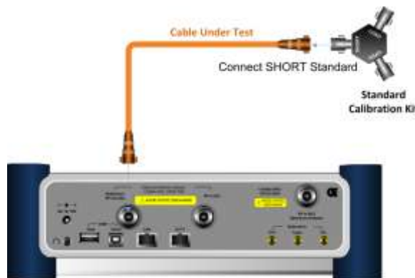
Figure 236 Connection for cable loss (1 port) measurement
