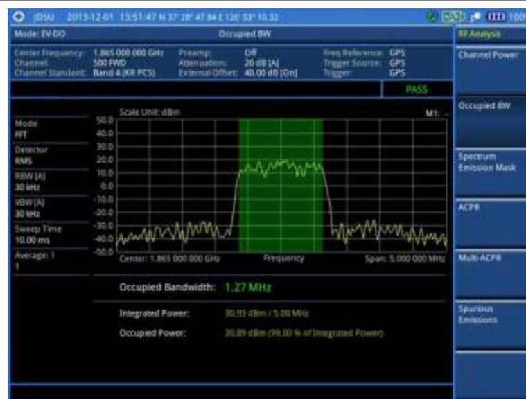
Figure 168 Occupied bandwidth measurement with EV-DO signal analyzer
