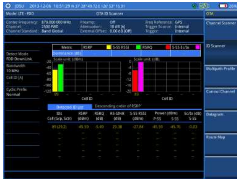
Figure 98 ID scanner measurement with LTE - FDD OTA signal analyzer
