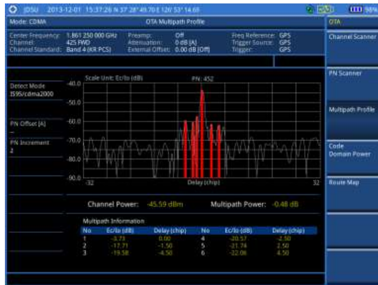
Figure 158 Multipath profile measurement with CDMA OTA signal analyzer
