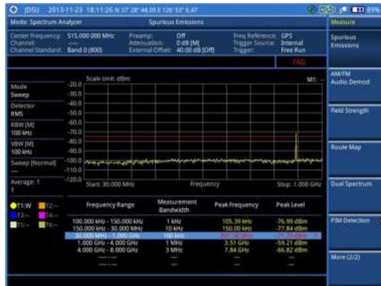
Figure 13 Spurious emissions measurement with spectrum analyzer
