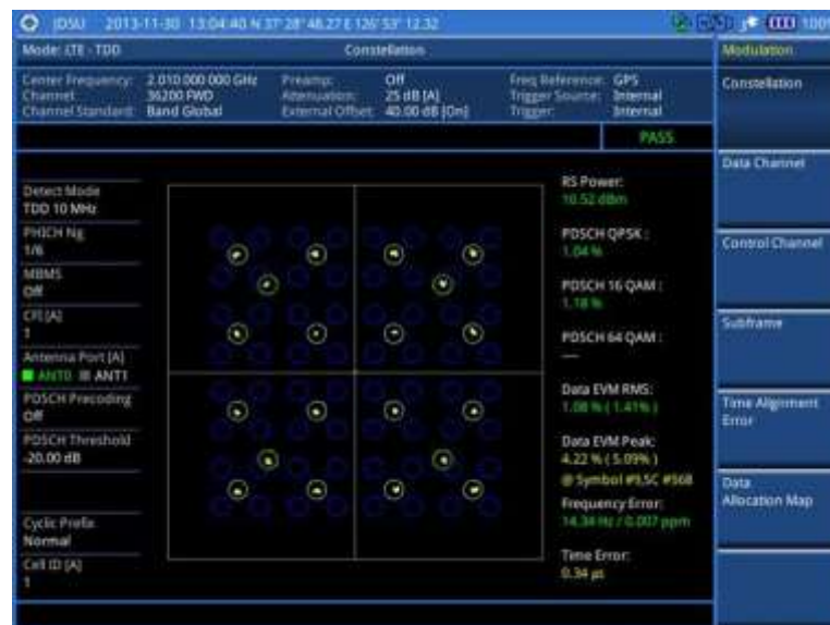
Figure 117 Constellation measurement with LTE - TDD signal analyzer
