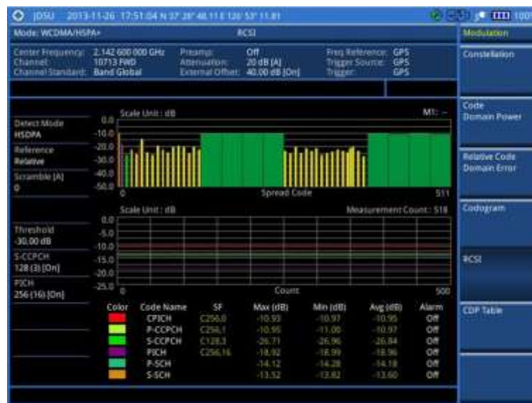
Figure 59 RCSI measurement with WCDMA/HSPA+ signal analyzer
