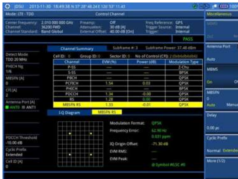
Figure 122 Control channel measurement with LTE - TDD signal analyzer (MBMS On)
