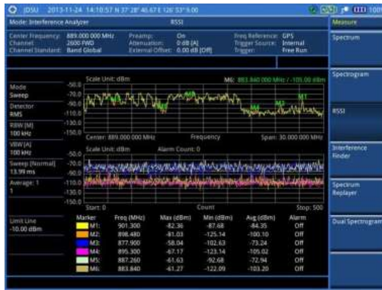
Figure 25 Interference measurement in RSSI
