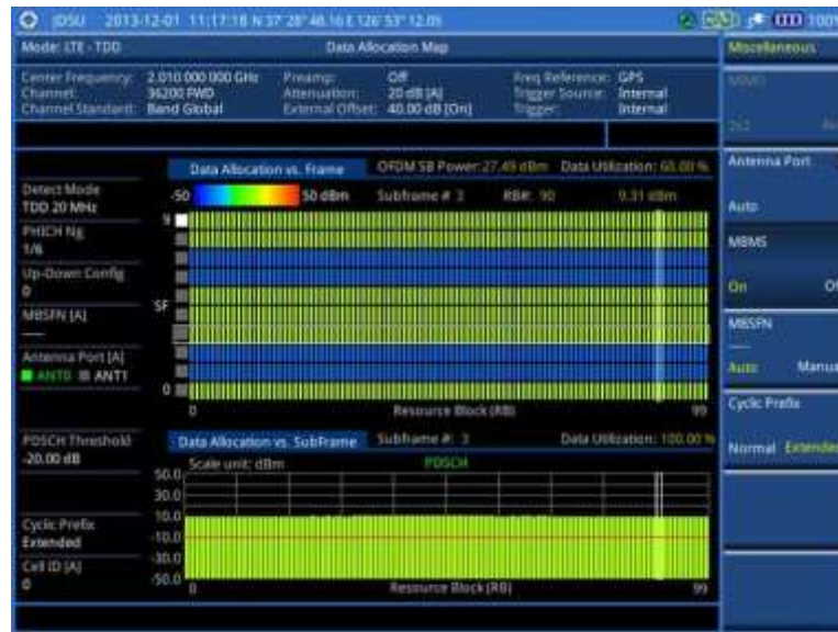
Figure 127 Data allocation map measurement with LTE - TDD signal analyzer (MBMS On)
