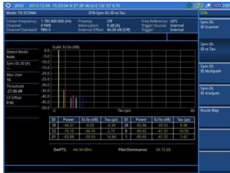
Figure 207 Sync-DL ID vs. Tau measurement with TD-SCDMA OTA signal analyzer
