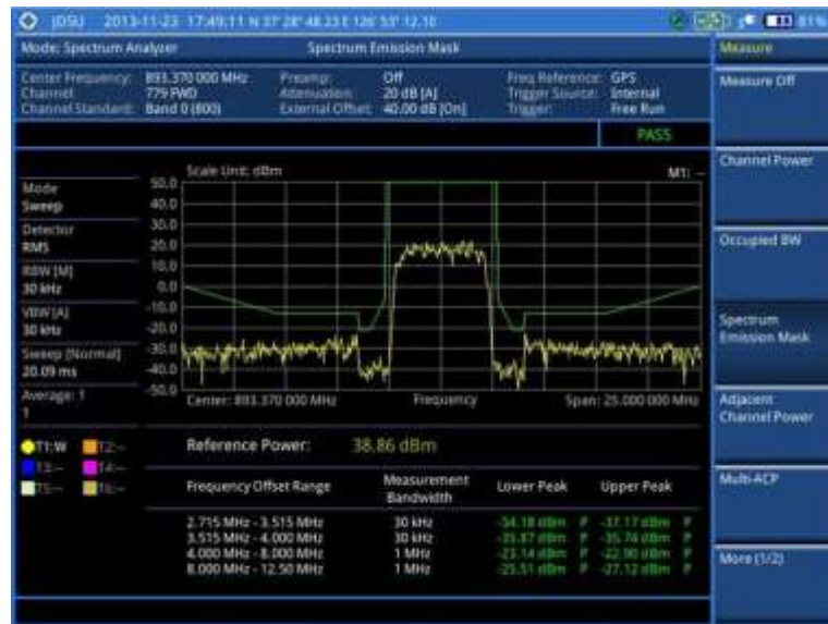
Figure 10 Spectrum emission mask measurement with spectrum analyzer
