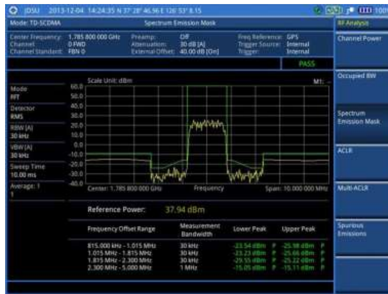
Figure 194 SEM measurement with TD-SCDMA signal analyzer
