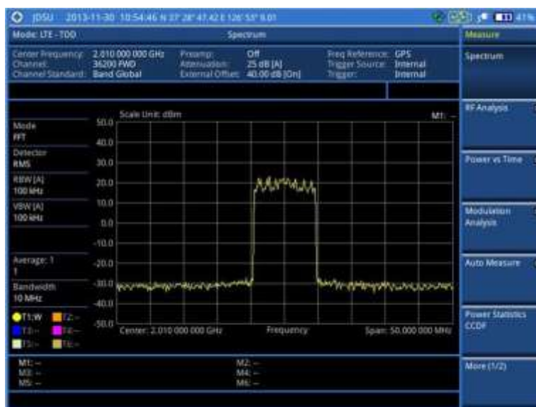
Figure 108 Spectrum measurement screen with LTE - TDD signal analyzer
