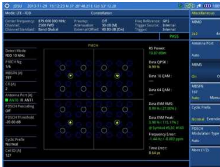
Figure 81 Constellation measurement with LTE - FDD signal analyzer (MBMS On)
