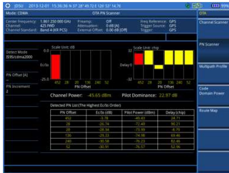
Figure 157 PN scanner measurement with CDMA OTA signal analyzer
