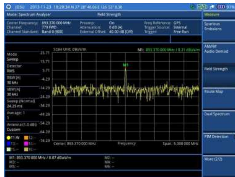
Figure 15 Field strength measurement with spectrum analyzer
