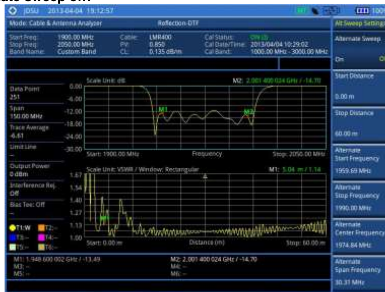
Figure 242 Reflection-DTF dual measurement
