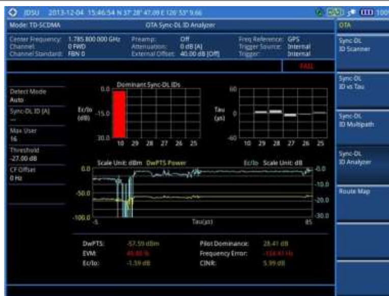
Figure 209 Sync-DL ID analyzer measurement with TD-SCDMA OTA signal analyzer
