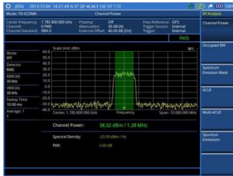
Figure 192 Channel power measurement with TD-SCDMA signal analyzer
