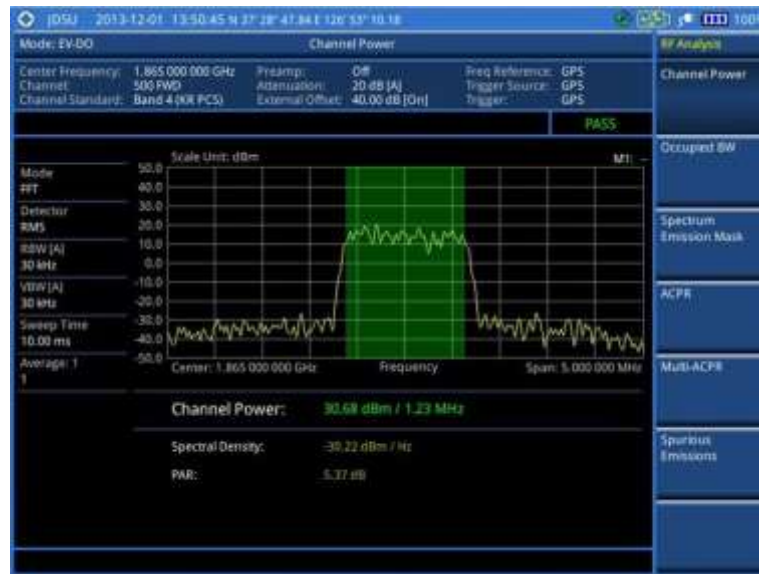
Figure 167 Channel power measurement with EV-DO signal analyzer
