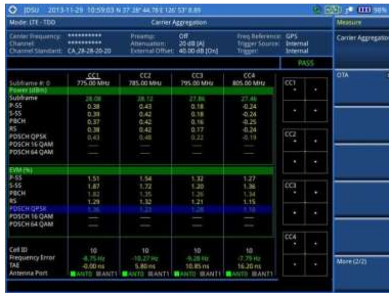
Figure 131 Carrier aggregation measurement with LTE - TDD signal analyzer (SA)
