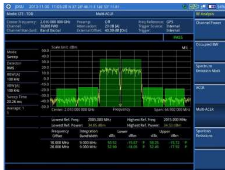
Figure 113 Multi-ACLR measurement with LTE - TDD signal analyzer
