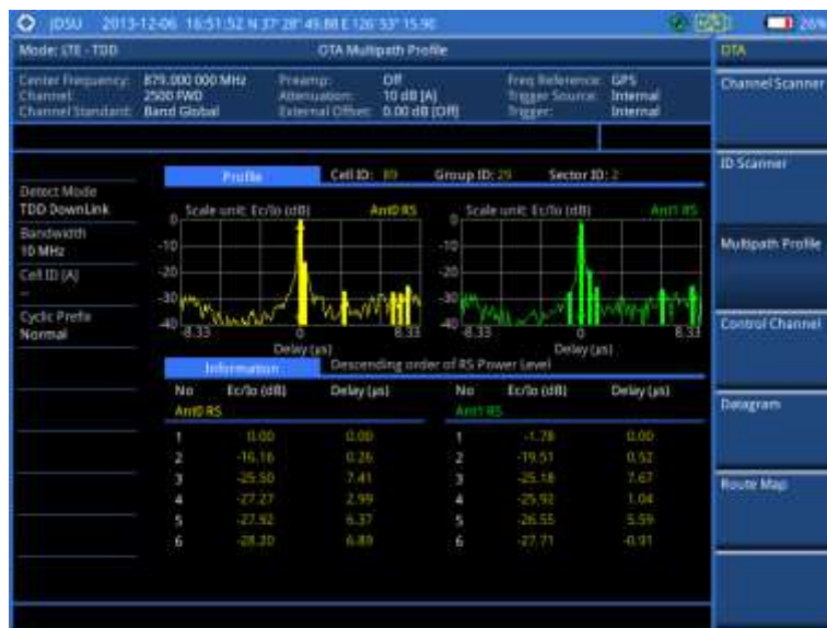
Figure 134 Multipath profile measurement with LTE - TDD OTA signal analyzer
