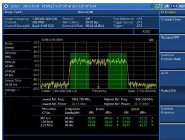
Figure 171 Multi-ACPR measurement with EV-DO signal analyzer
