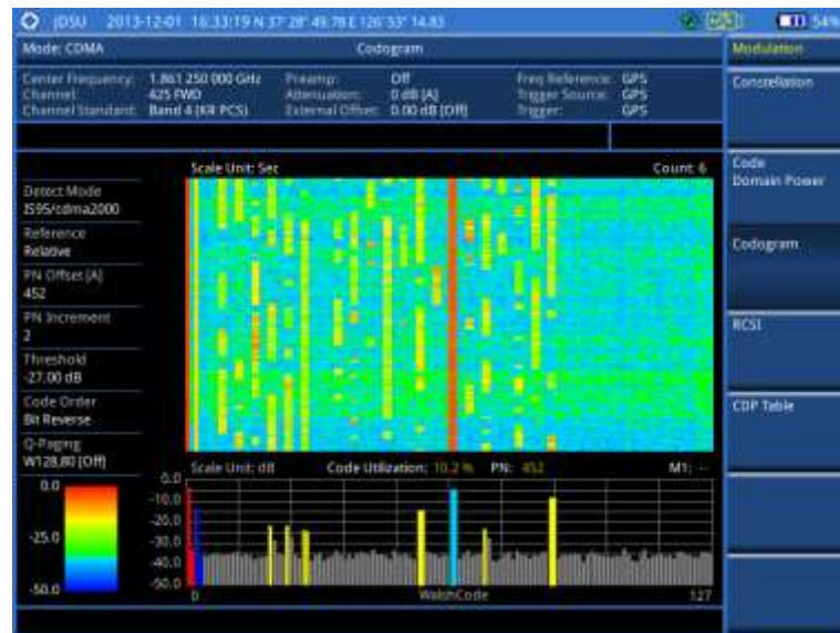
Figure 152 Codogram in full view with CDMA signal analyzer
