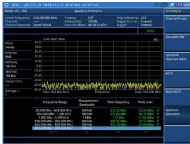
Figure 78 Spurious emissions measurement with LTE - FDD signal analyzer
