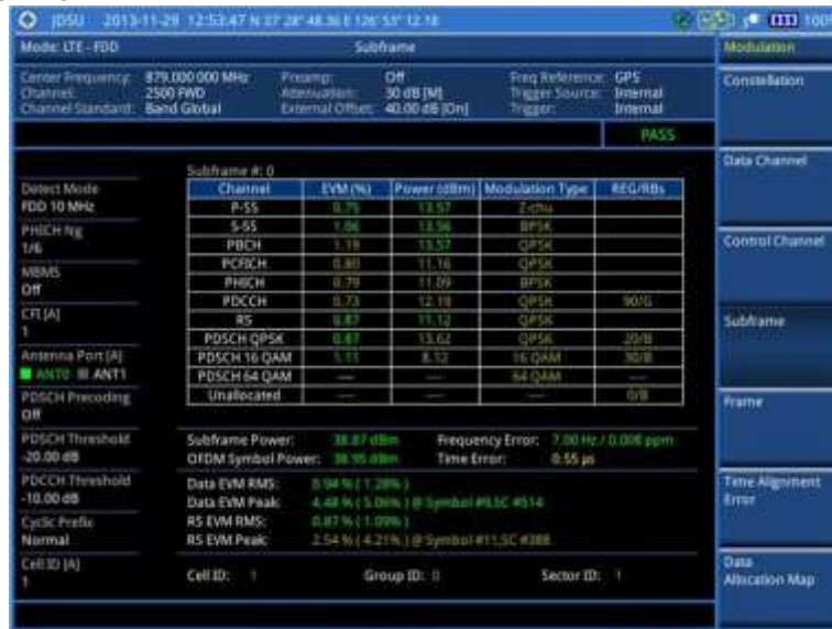
Figure 86 Subframe measurement with LTE - FDD signal analyzer
