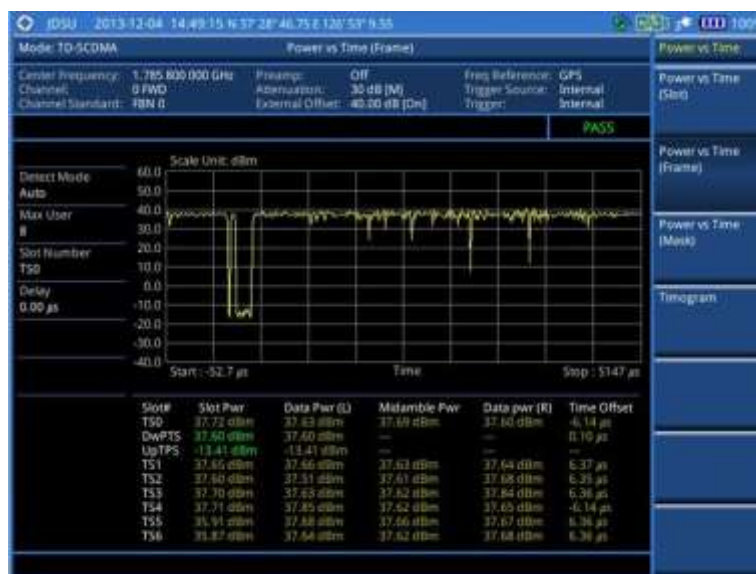
Figure 199 Power vs. time (frame) measurement with TD-SCDMA signal analyzer
