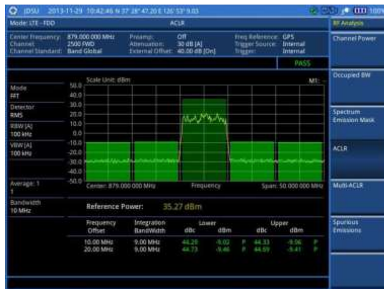
Figure 76 ACLR measurement with LTE - FDD signal analyzer
