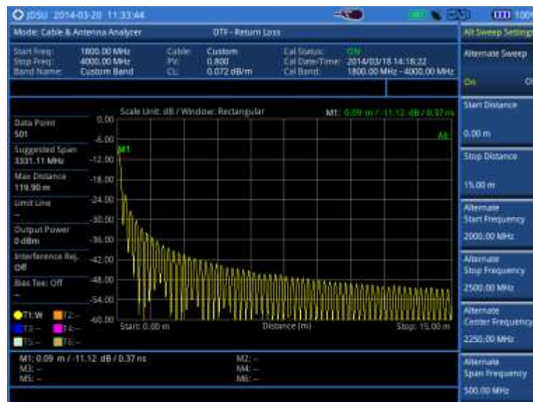
Figure 241 DTF measurement with the alternate sweep on
