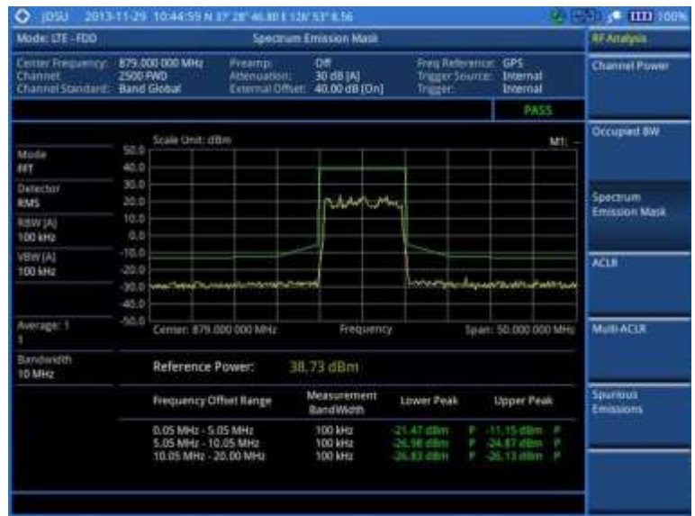
Figure 75 SEM measurement with LTE - FDD signal analyzer
