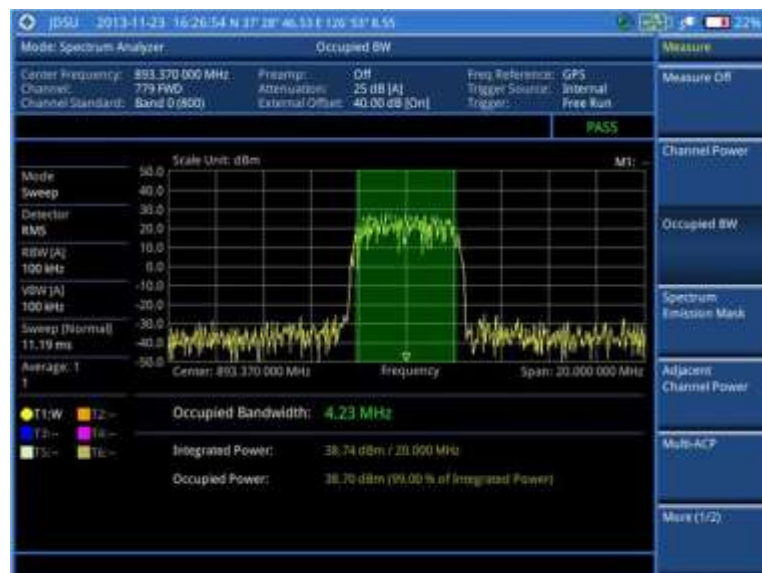
Figure 9 Occupied bandwidth measurement with spectrum analyzer
