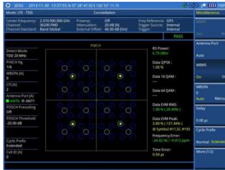
Figure 118 Constellation measurement with LTE - TDD signal analyzer (MBMS On)
