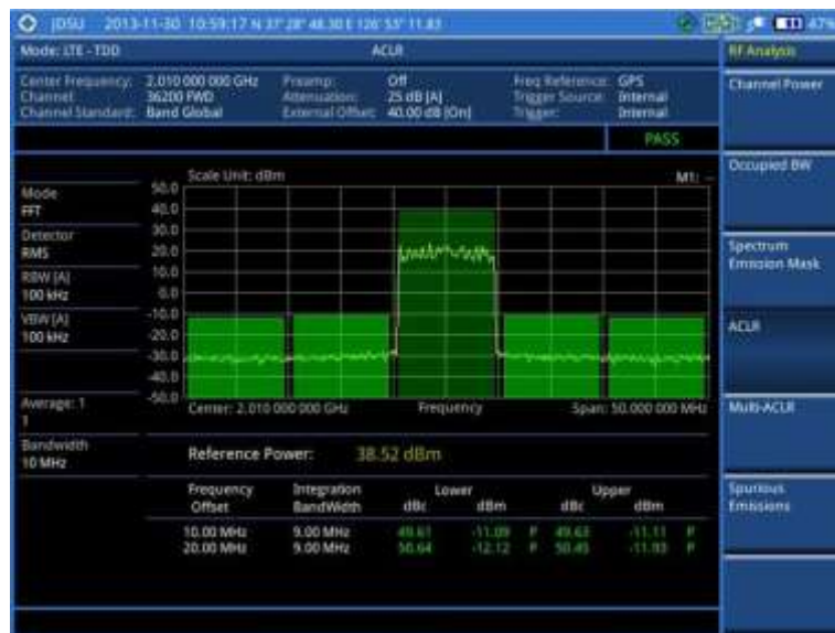
Figure 112 ACLR measurement with LTE - TDD signal analyzer
