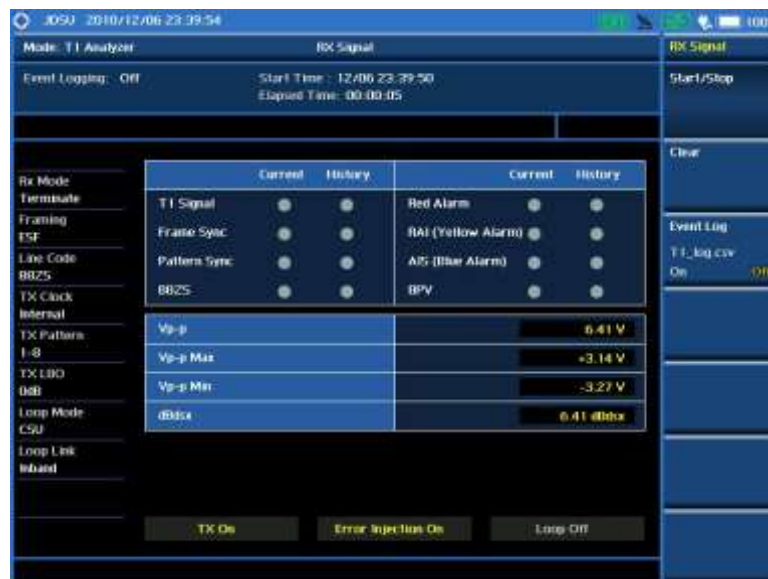
Figure 263 T1 RX signal testing
