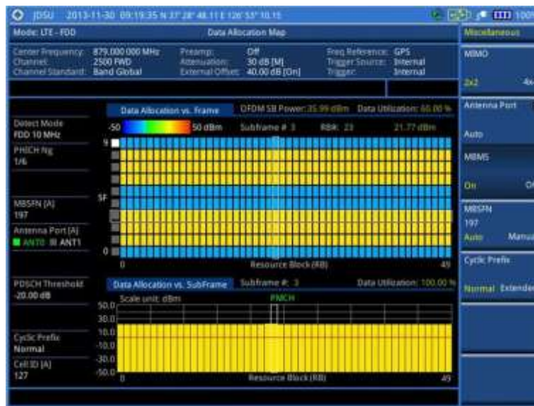
Figure 92 Data allocation map measurement with LTE - FDD signal analyzer (MBMS On)
