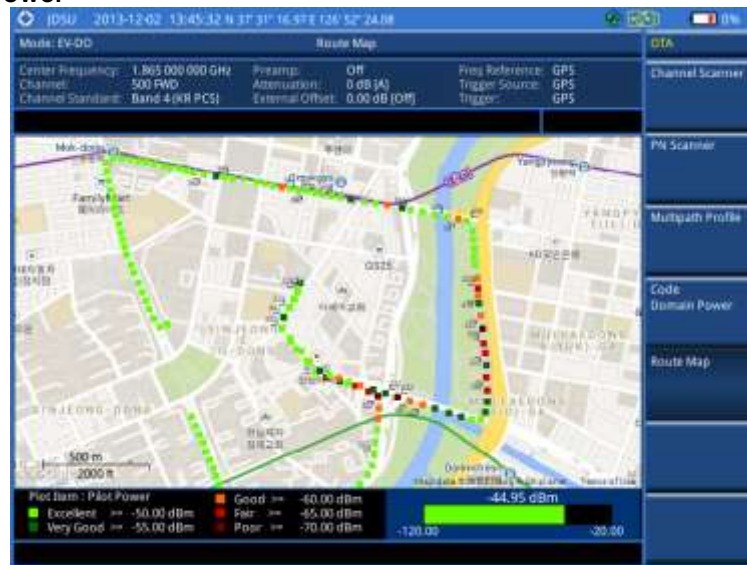
Figure 185 Route map measurement with EV-DO OTA signal analyzer
