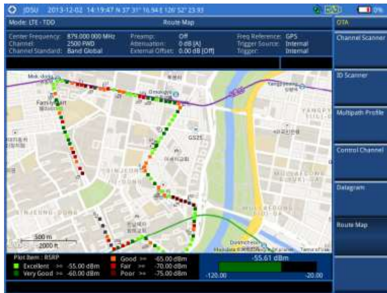
Figure 137 Route map measurement with LTE - TDD OTA signal analyzer
