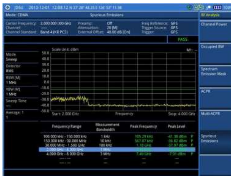
Figure 149 Spurious emissions measurement with CDMA signal analyzer
