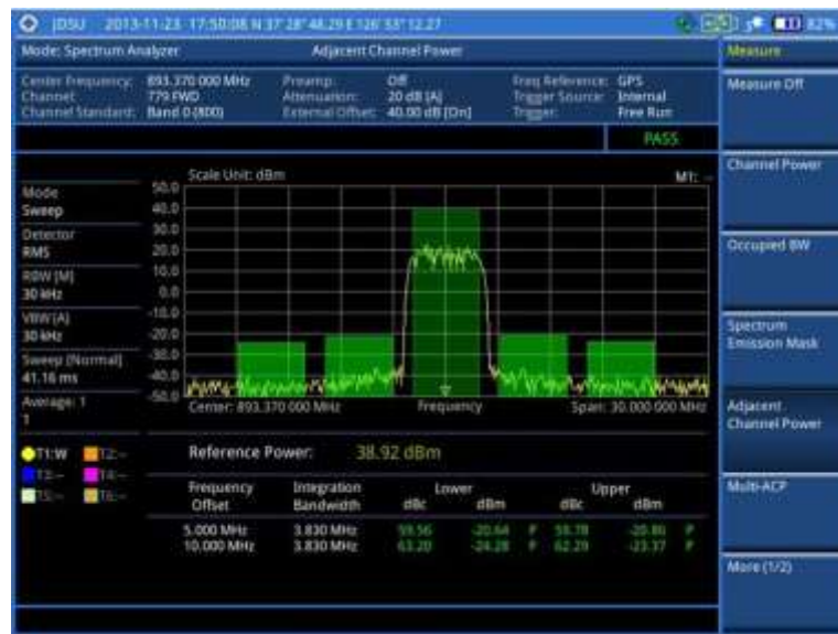
Figure 11 Adjacent channel power measurement with spectrum analyzer
