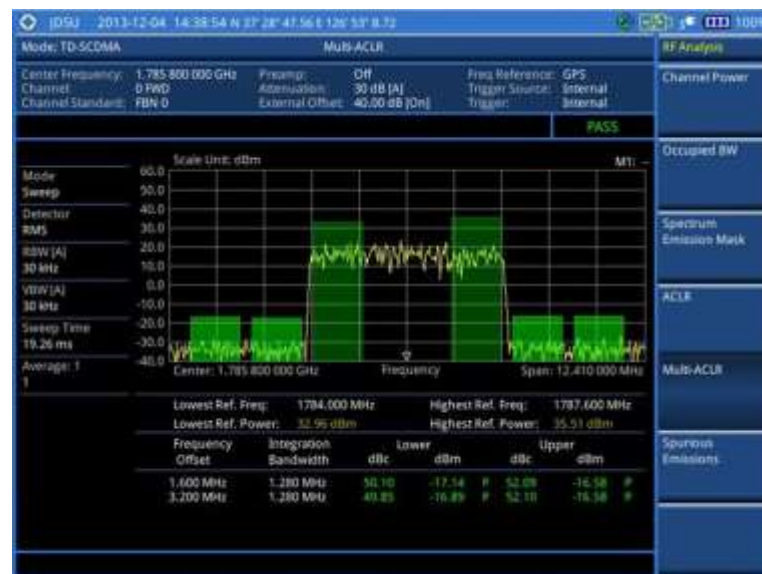
Figure 196 Multi-ACLR measurement with TD-SCDMA signal analyzer
