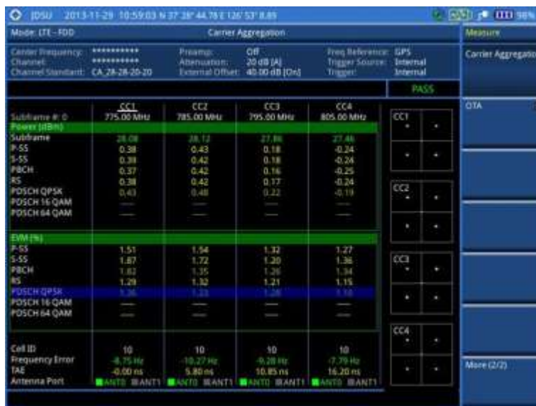
Figure 96 Carrier aggregation measurement with LTE - FDD signal analyzer (SA)
