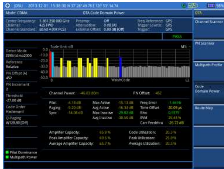
Figure 159 Code domain power measurement with CDMA OTA signal analyzer
