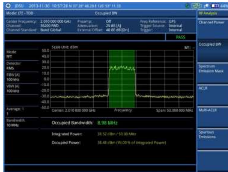
Figure 110 Occupied bandwidth measurement with LTE - TDD signal analyzer
