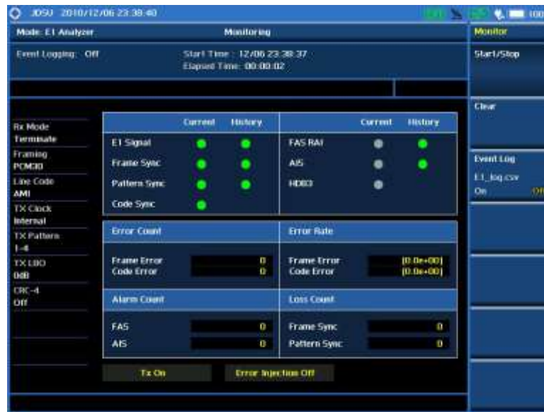
Figure 254 E1 transmission monitoring for framing PCM30
