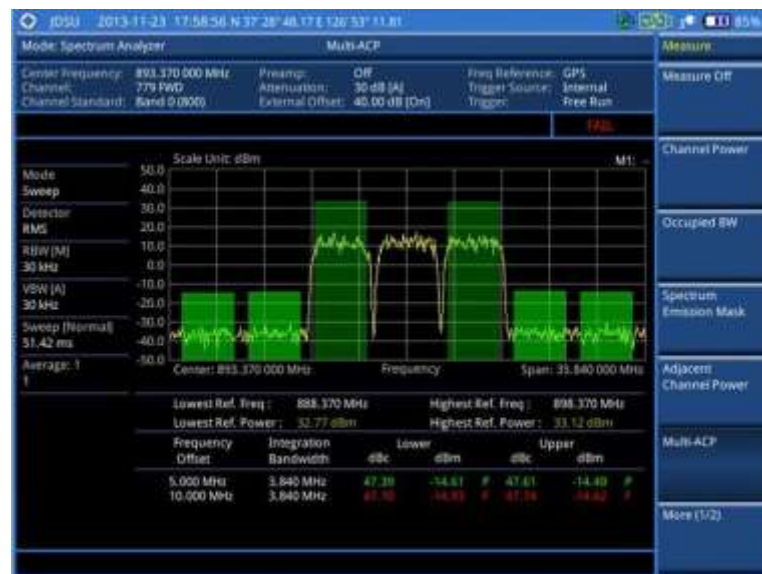
Figure 12 Multi-ACP measurement with spectrum analyzer
