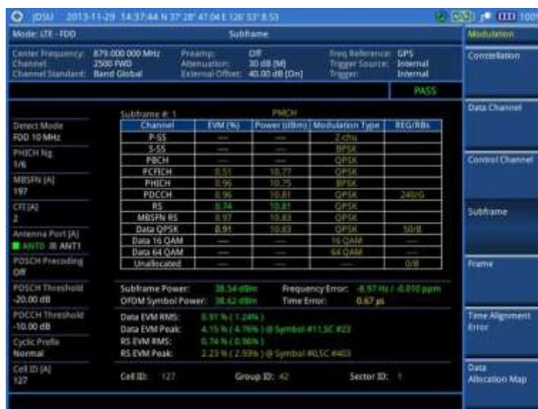
Figure 87 Subframe measurement with LTE - FDD signal analyzer (MBMS On)
