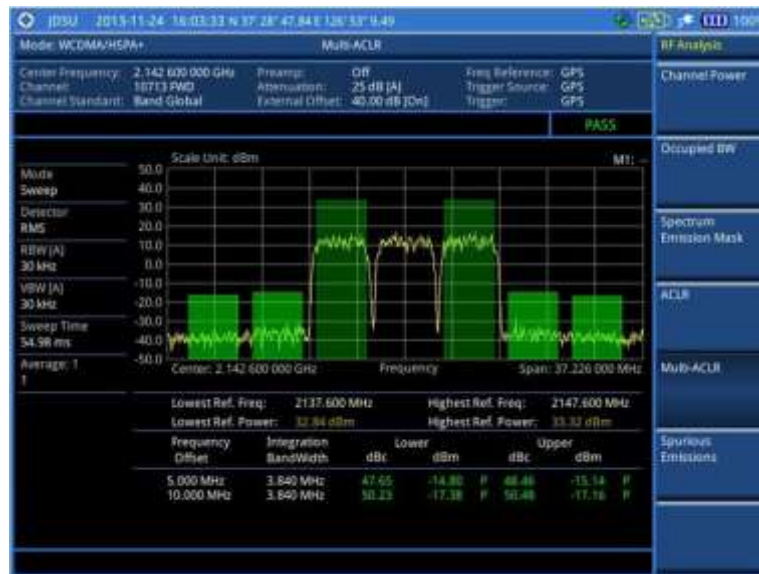
Figure 53 Multi-ACLR measurement with WCDMA/HSPA+ signal analyzer
