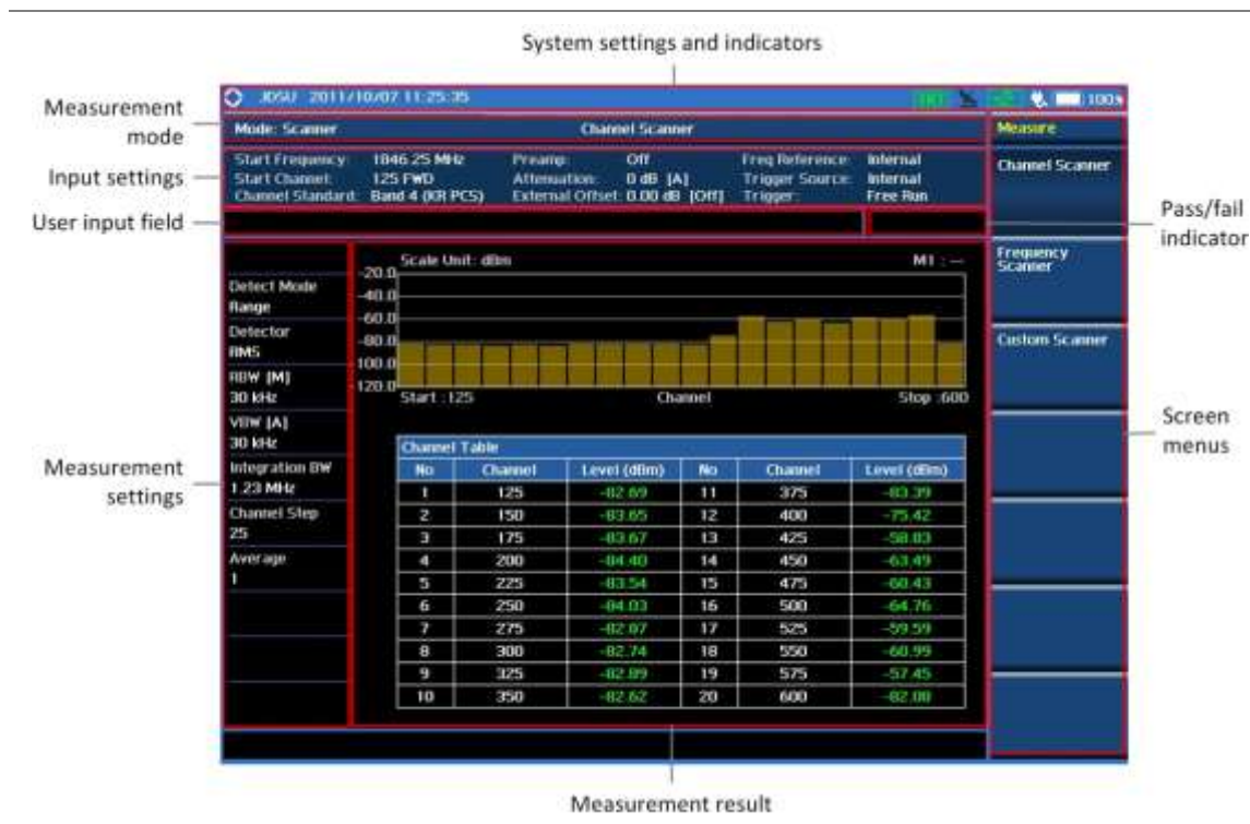
Figure 265 Channel scanner screen
