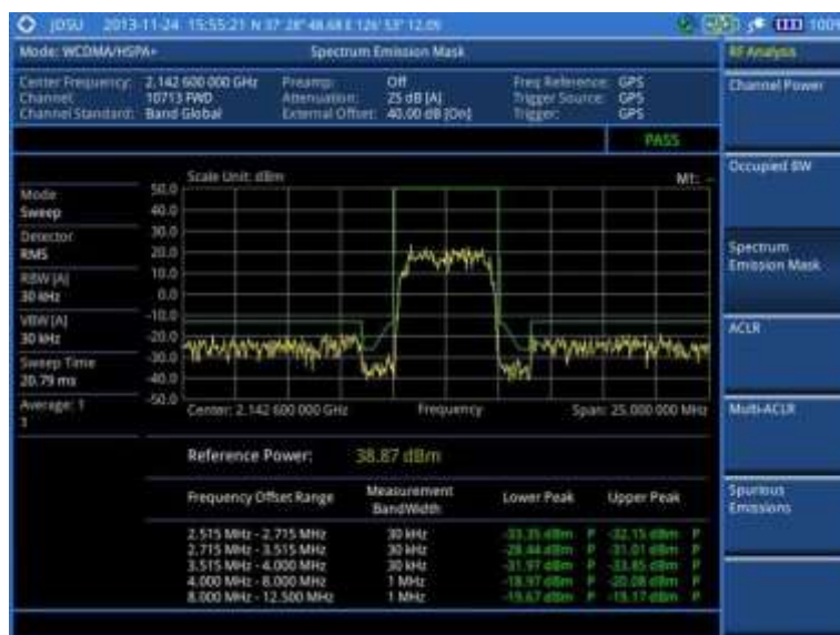
Figure 51 SEM measurement with WCDMA/HSPA+ signal analyzer
