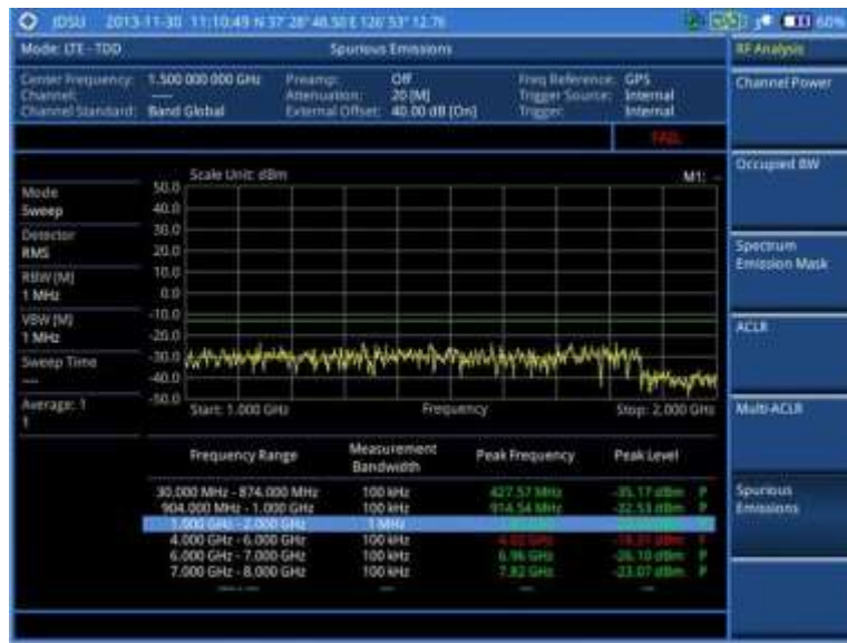
Figure 114 Spurious emissions measurement with LTE - TDD signal analyzer
