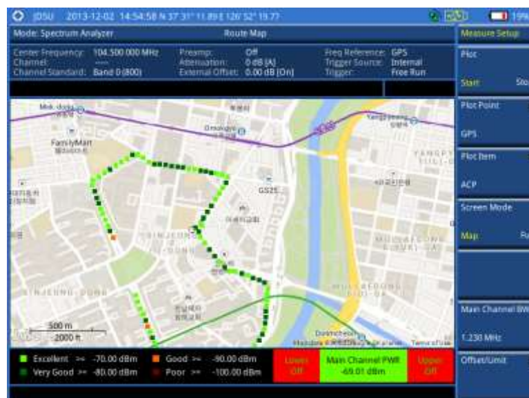
Figure 16 Route map measurement screen with GPS
