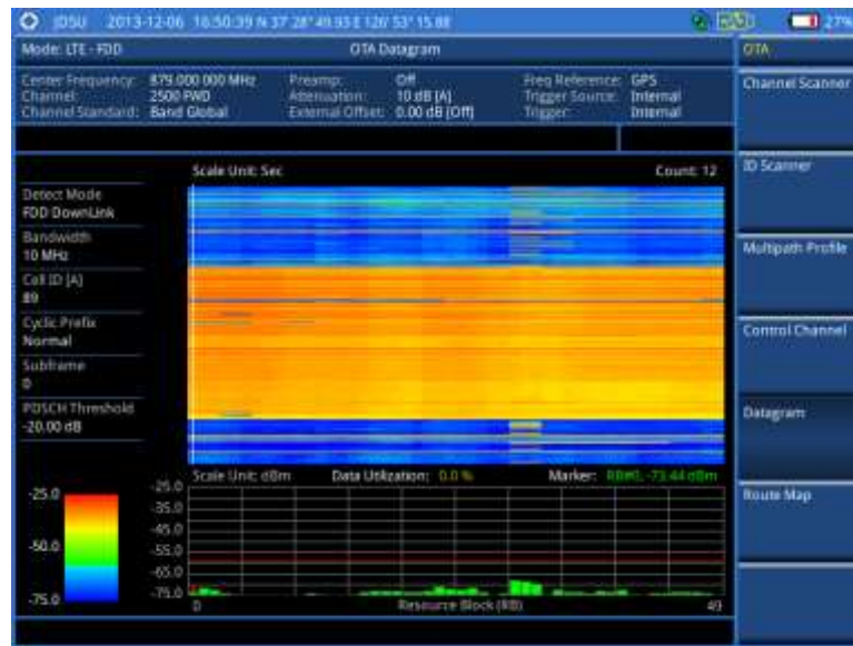
Figure 101 Datagram measurement with LTE - FDD signal analyzer
