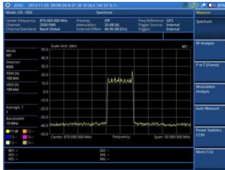
Figure 72 Spectrum measurement screen with LTE - FDD signal analyzer
