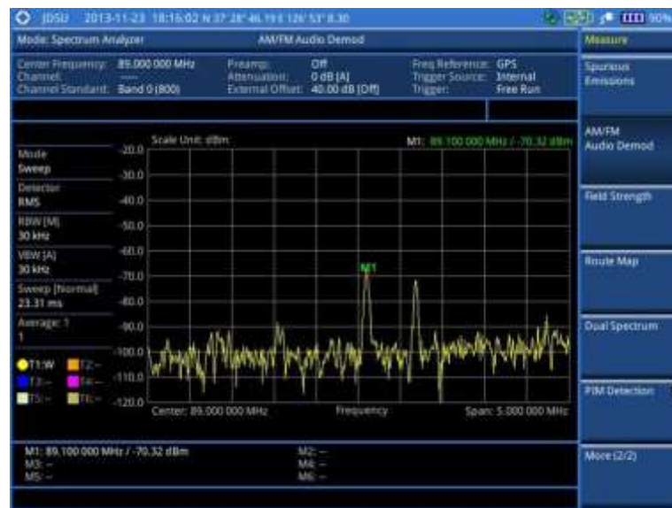
Figure 14 AM/FM audio demodulation with spectrum analyzer
