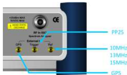
Figure 47 Connection ports for external reference clock
