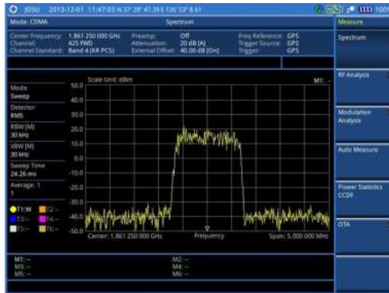
Figure 143 Spectrum measurement screen with CDMA signal analyzer
