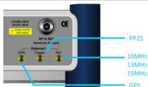
Figure 71 Connection ports for external reference clock
