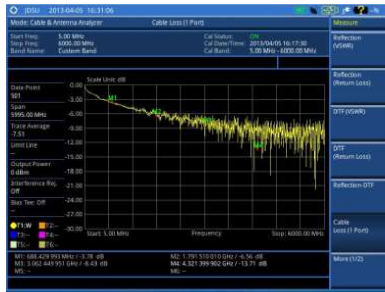
Figure 243 Cable loss (1 port) measurement
