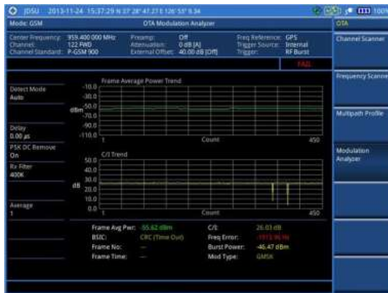
Figure 42 Modulation analyzer measurement with GSM OTA signal analyzer
