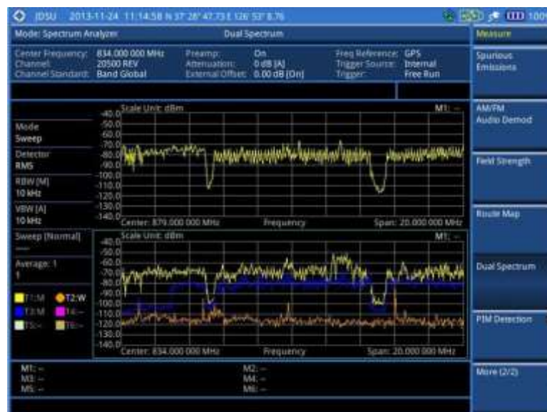
Figure 17 Dual spectrum measurement with spectrum analyzer
