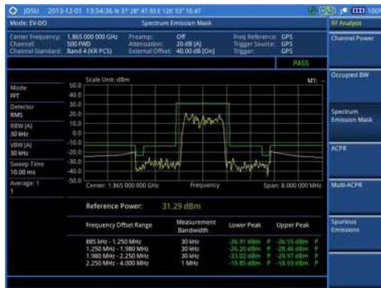
Figure 169 SEM measurement with EV-DO signal analyzer
