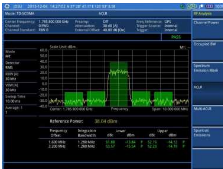
Figure 195 ACLR measurement with TD-SCDMA signal analyzer
