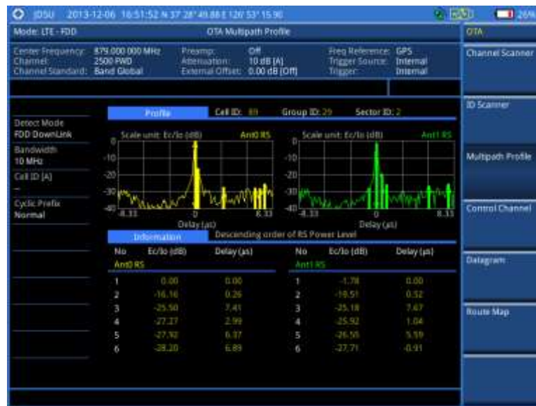
Figure 99 Multipath profile measurement with LTE - FDD OTA signal analyzer
