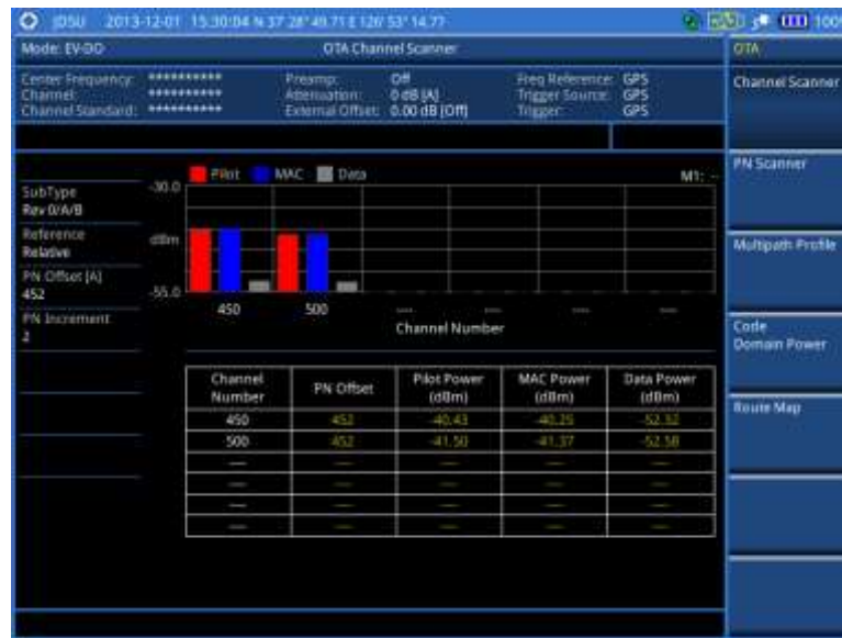
Figure 181 Channel scanner measurement with EV-DO OTA signal analyzer
