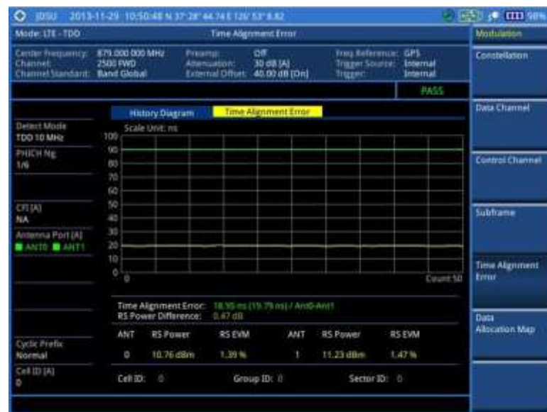
Figure 125 Time alignment error measurement with LTE - TDD signal analyzer
