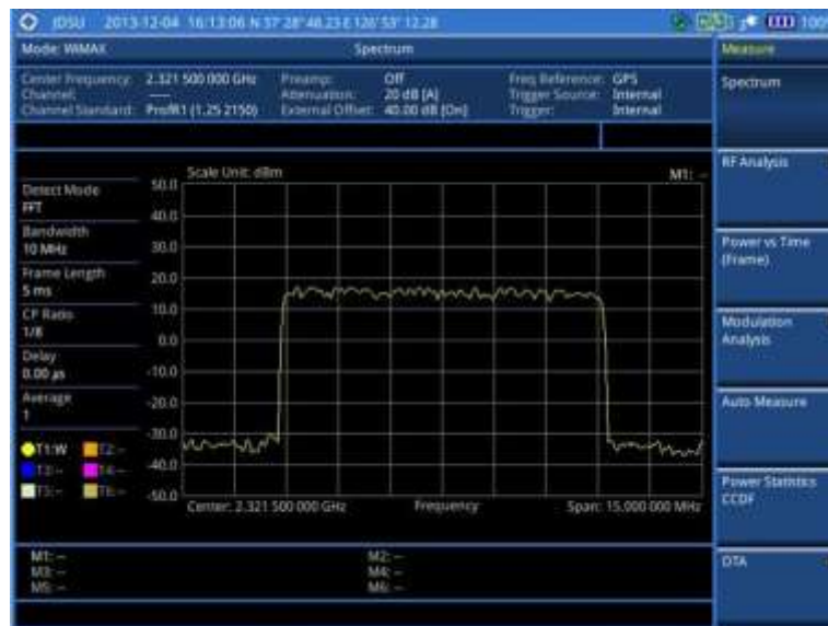
Figure 216 Spectrum measurement screen with Mobile WiMAX signal analyzer
