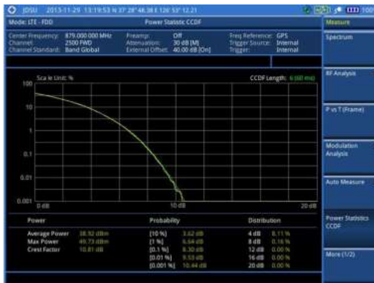
Figure 94 CCDF measurement with LTE - FDD signal analyzer
