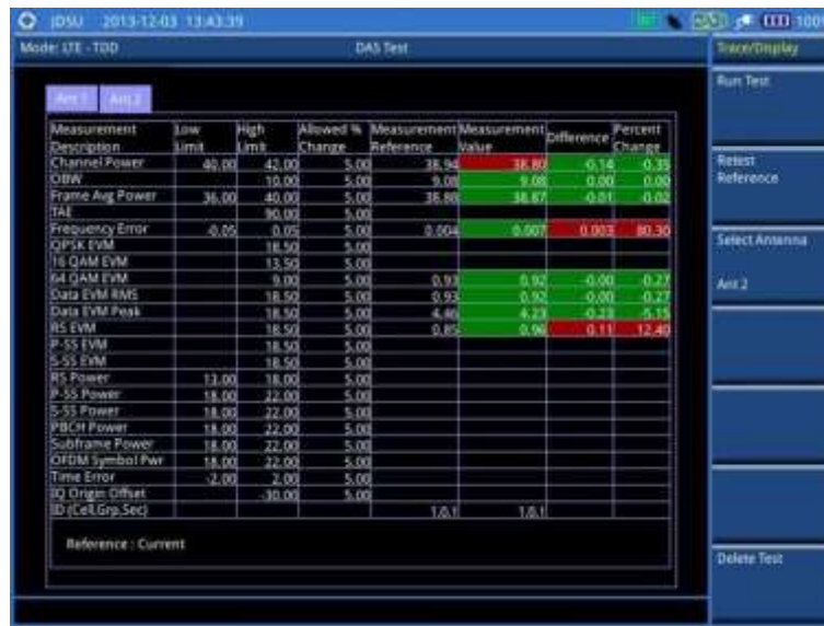
Figure 128 DAS measurement with LTE - TDD signal analyzer
