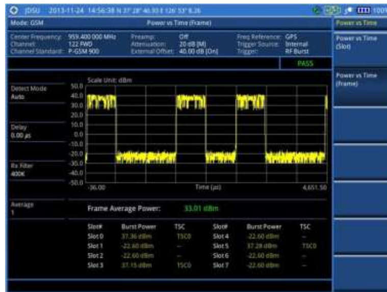
Figure 37 Power vs. time (frame) measurement with GSM signal analyzer
