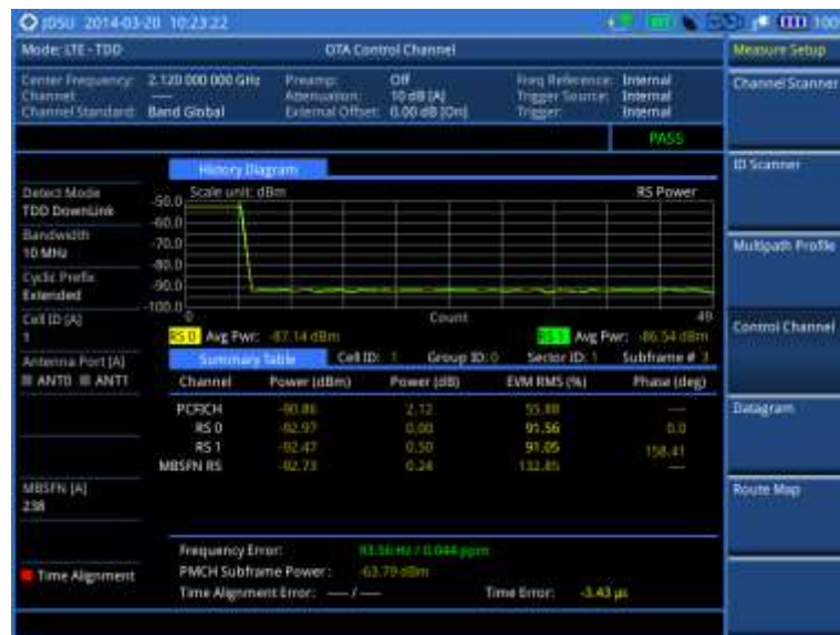
Figure 135 Control channel measurement with LTE - TDD OTA signal analyzer
