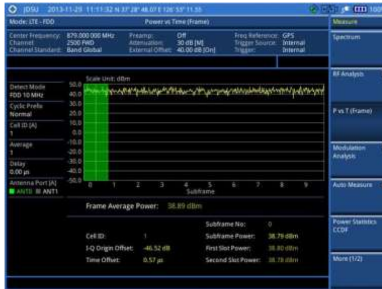
Figure 79 Power vs. time (frame) measurement with LTE – FDD signal analyzer
