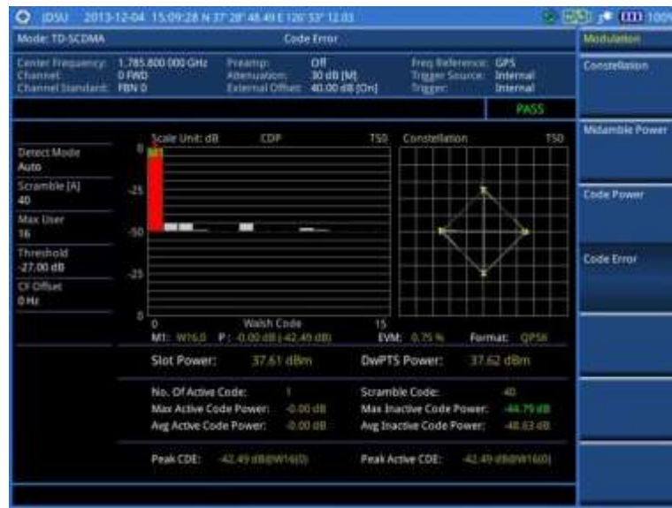
Figure 205 Code error measurement with TD-SCDMA signal analyzer
