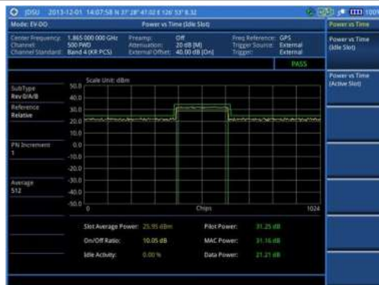
Figure 173 Power vs. time (idle slot) measurement with EV-DO signal analyzer
