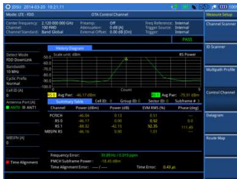
Figure 100 Control channel measurement with LTE - FDD OTA signal analyzer
