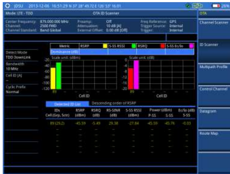
Figure 133 ID scanner measurement with LTE - TDD OTA signal analyzer
