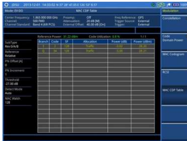
Figure 179 MAC CDP Table measurement with EV-DO signal analyzer
