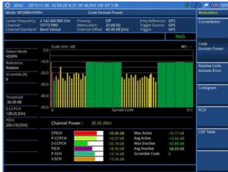
Figure 56 Code domain power measurement with WCDMA/HSPA+ signal analyzer
