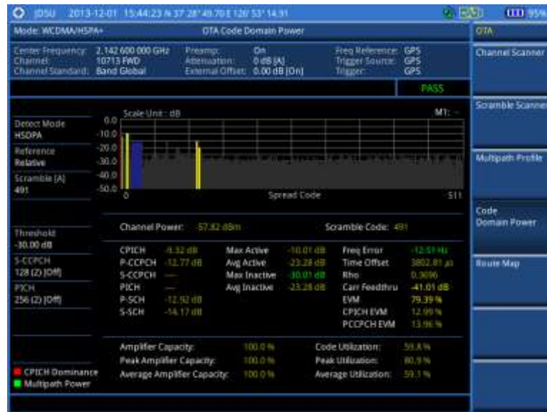
Figure 65 Code domain power measurement with WCDMA/HSPA+ OTA signal analyzer
