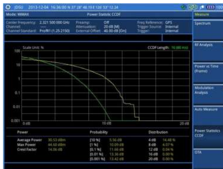
Figure 226 CCDF measurement with Mobile WiMAX signal analyzer
