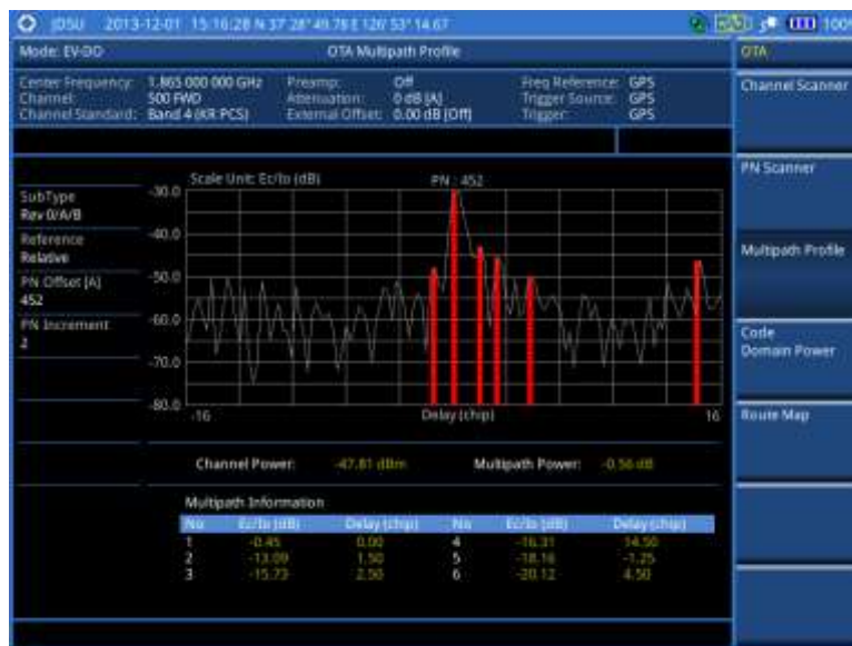
Figure 183 Multipath profile measurement with EV-DO OTA signal analyzer
