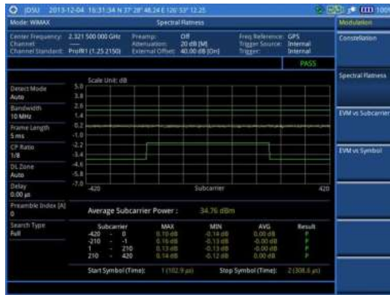
Figure 223 Spectral flatness measurement with Mobile WiMAX signal analyzer
