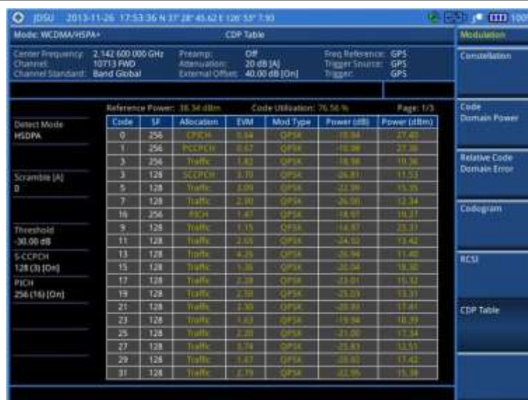
Figure 60 CDP Table measurement with WCDMA/HSPA+ signal analyzer
