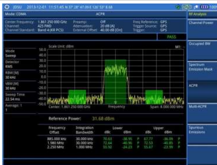
Figure 147 ACPR measurement with CDMA signal analyzer
