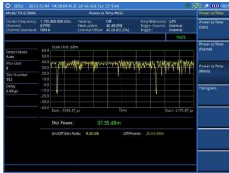
Figure 200 Power vs. time (mask) measurement with TD-SCDMA signal analyzer
