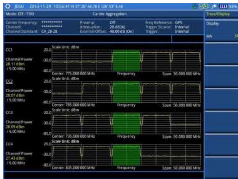
Figure 131 Carrier aggregation measurement with LTE - TDD signal analyzer (SA)
