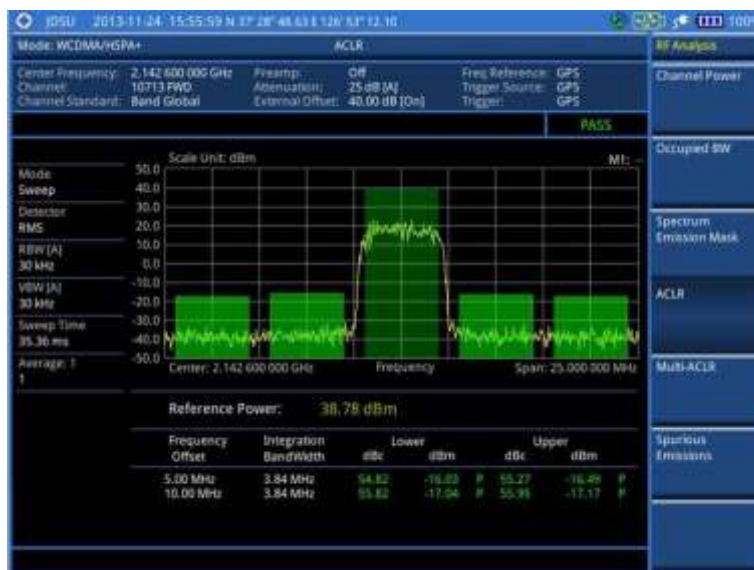
Figure 52 ACLR measurement with WCDMA/HSPA+ signal analyzer
