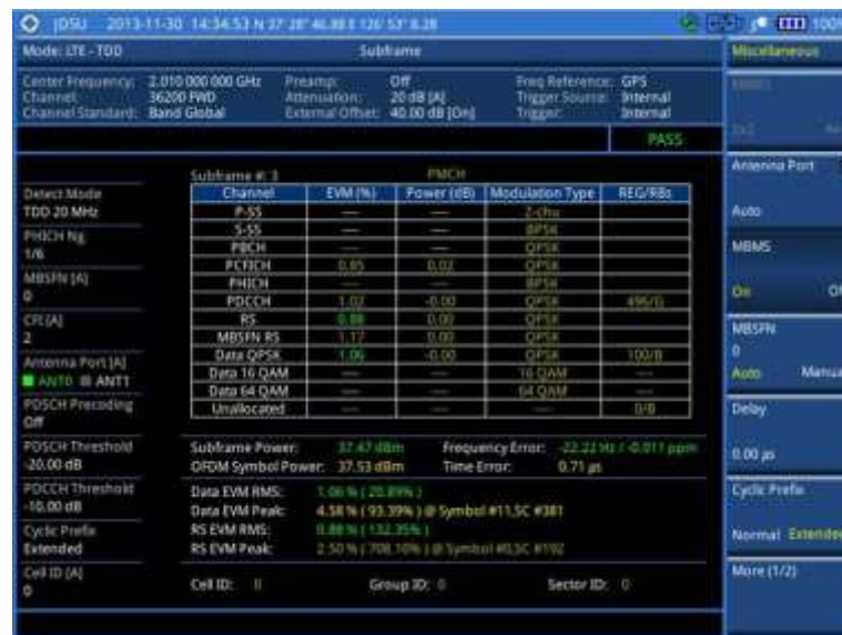
Figure 124 Subframe measurement with LTE - TDD signal analyzer (MBMS On)
