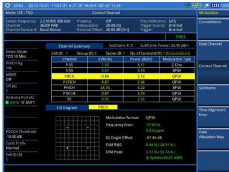
Figure 122 Control channel measurement with LTE - TDD signal analyzer (MBMS On)
