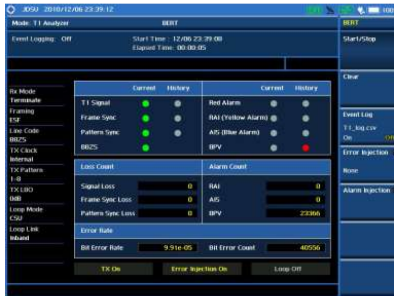
Figure 262 T1 BERT testing
