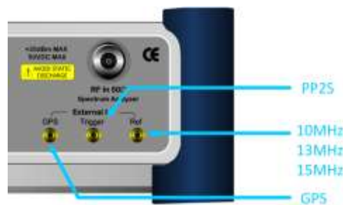
Figure 165 Connection ports for external reference clock
