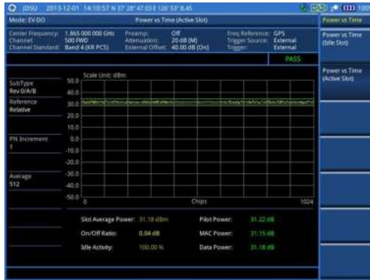
Figure 174 Power vs. time (active slot) measurement with EV-DO signal analyzer
