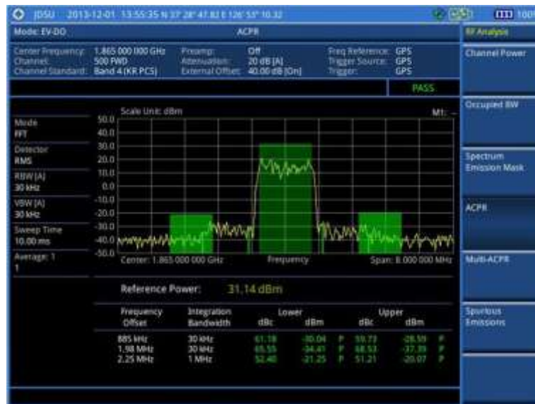
Figure 170 ACPR measurement with EV-DO signal analyzer
