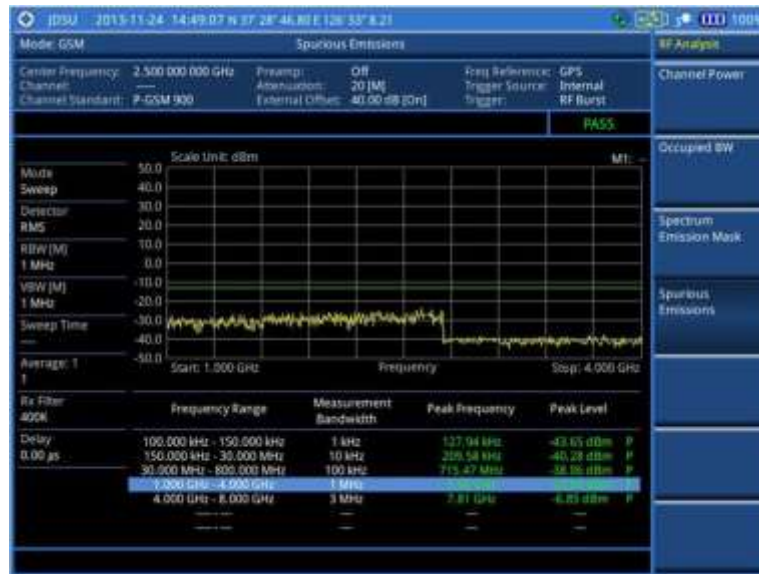
Figure 35 Spurious emissions measurement with GSM signal analyzer
