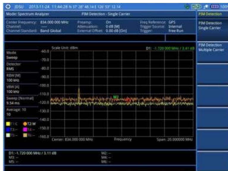
Figure 18 PIM detection for single carrier
