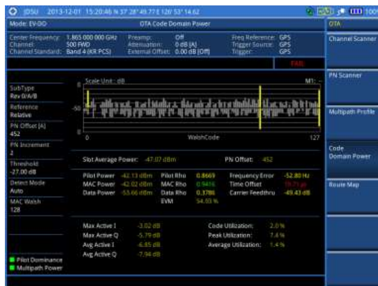
Figure 184 Code domain power measurement with EV-DO OTA signal analyzer
