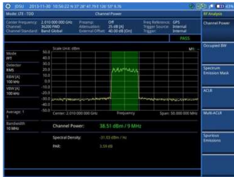
Figure 109 Channel power measurement with LTE - TDD signal analyzer
