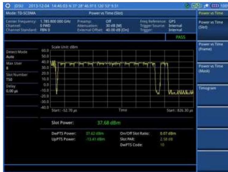
Figure 198 Power vs. time (slot) measurement with TD-SCDMA signal analyzer
