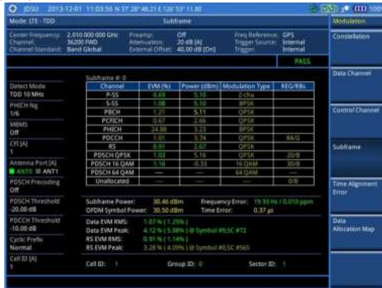
Figure 123 Subframe measurement with LTE - TDD signal analyzer
