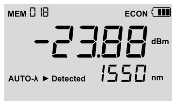
Fig. 5 Display in Auto- \lambda mode showing one detected wavelength and their power levels.
