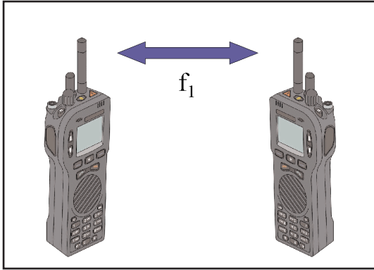
Figure 1.0 shows conventional communication between two radios using simplex operation.
