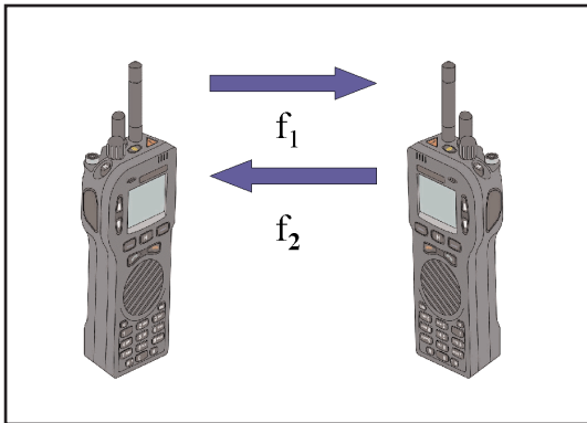
Figure 2.0 Two-way radio communication using duplex operation
