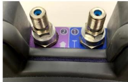
RF ports with collars between the F-81 barrel-connectors and ONX body
