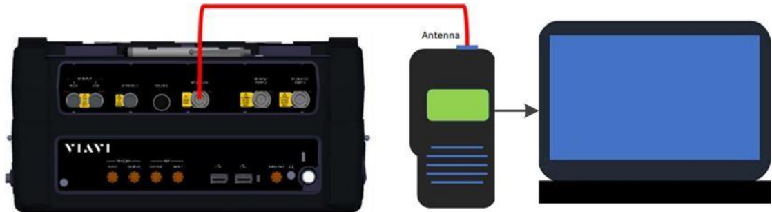
Figure 3-2 NXDN Receiver Sensitivity Test Setup Diagram
