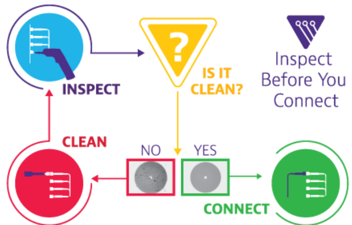
Figure 11: Inspect Before You Connect
