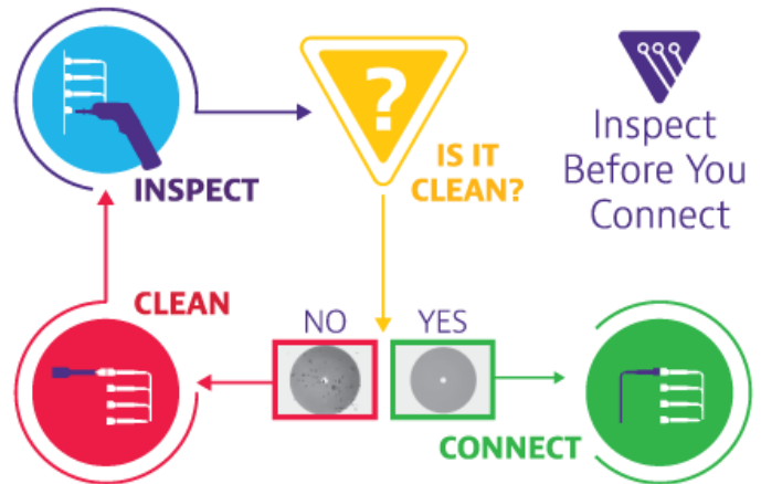
Figure 12: Inspect Before You Connect
